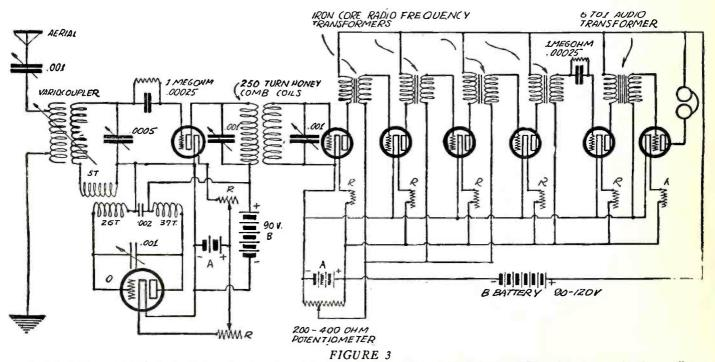
A wiring diagram of the super-heterodyne receiver, given in the November, 1923, RADIO AGE, with changes in the oscillator and modulator circuits, which have been found more efficient.
