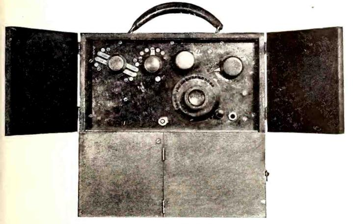
FRONT OF CABINET Figure 2. The portable receiver, with hinged doors opened to show panel arrangement.
