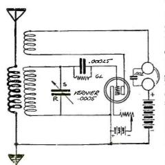
FIGURE 6 A wiring diagram for the honeycomb coils shown in Figure 3, Illustration 3.
