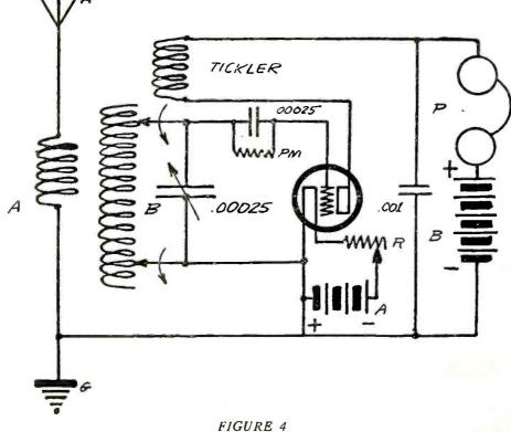
The aperiodically coupled single circuit receiver. A condenser of 11 or 23 plates should be connected across the two switch levers for the best possible results
