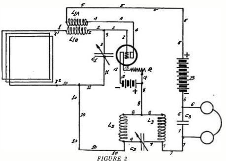
The wiring diagram of the Traveling Men's receiver.
