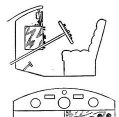
Figure 2. Sketches showing method of mounting receiver under the dash of
