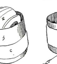
Figure 1c. Arrangement of the coupler and plate coils.
