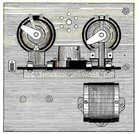
Figure 2. The back panel layout of the simple Sure Fire Reflex Receiver.
