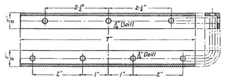
Figure 5. The bracket supporting the shelf is drilled in the manner shown herewith for the best mounting arrangement.
