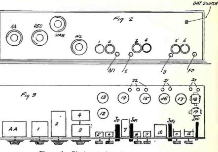
Figure 1b. The layout of the Superdyne receiver.
