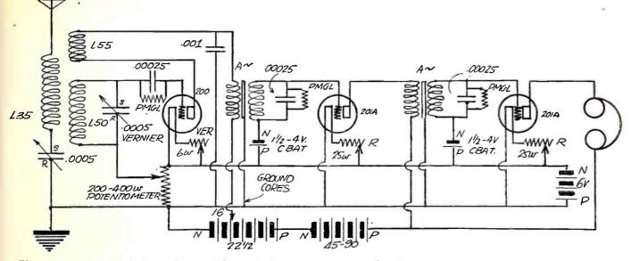
Figure 2. A diagram of the receiver used by T. J. Kennedy in his record breaking receptions. The secondaries of the audio transformers are shunted by a .00025 MF condenser and a variable pencil mark grid leak.
