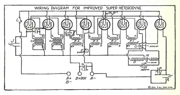
possible to make changes in the nature of the matter between the elements. However, it is possible to reduce the capacity of the grid and plate by reducing the frequency or wave length of the current in the plate and grid, and this is exactly what is done in the super-heterodyne circuit.
