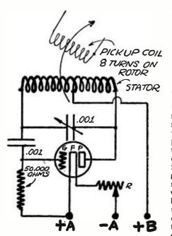
Figure 2. A diagram of the Hartley Oscillator.
