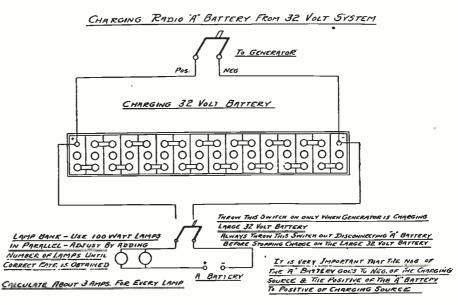
Figure 3. You can charge your A battery just like a regular charging station in the manner shown herewith. The charging is done at the same time as the household batteries are recharged. The A battery should not be charged separately.
