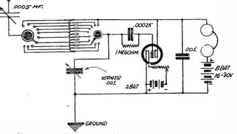
Figure 4. The FT circuit as revised by Mr. Baumgardner of Chicago. He finds this circuit very selective, and extremely sensitive to long distance stations.
