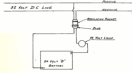
DETERMINE POLARITY OF LINE BY PLACING CHARGING LEADS IN A GLASS OF WATER & BYBBLES WILL ARISE FROM NEG LEAD IT IS VERY IMPORTANT THAT THE NEG. OF THE BATTERY CONNECTS TO THE NEG. OF THE CHARGING LINE & THE POSITIVE OF THE BATTERY TO THE POS OF THE CHARGING LINE
