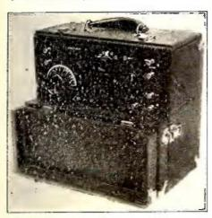
The portable is a regenerative detector and one-stage audio amplification outfit in a strong leatherette covered and nickel trimmed portable cabinet.
