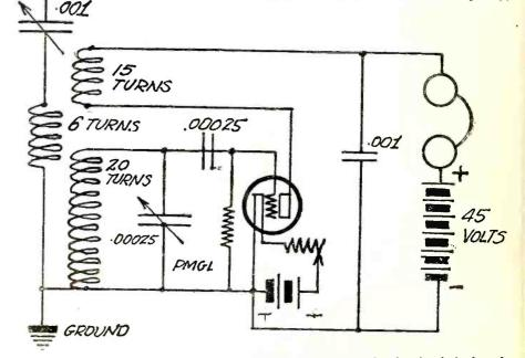
Figure 1. A diagram of a short wave receiver adapted to the signals of the broadcast relay stations. Often signals can be easily heard and distinguished on the shorter waves when not even the main wave can be heard.
