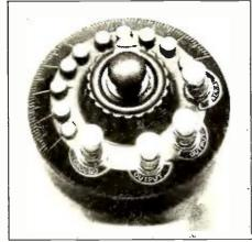
A top view of the "Dial Crystal Receiver" showing the arrangement of the taps, binding posts and illustrating the manner in which the vernier knob of the condenser dial is used as the switch knob to vary the inductance.
