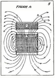
Figure 5. Showing how in this case all lines énter from the inside and pass out, producing maximum current in coil 2 by induction. This is the effect you obtain when your variocoupler is set at maximum.
