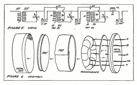
the metal box so that the unit may be fastened to the end plate of the tuning condenser. The bottom and sides are lined with felt (be generous) and the transformer windings are put into place.
