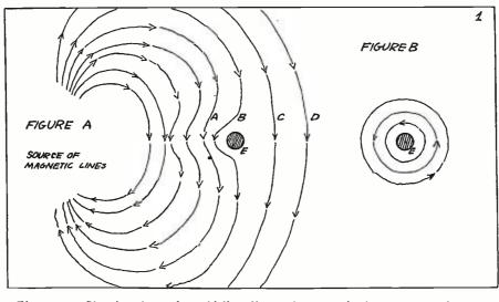
Figure 1. Showing how the whirling lines of magnetic force are made to cut through a conductor.
