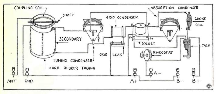
Circuit diagram of the Ultra-Audion receiver. There aren't many parts to assemble and the circuit is simple in operation. Special features are the antenna coupling coil, the low capacity grid condenser, the absorption condenser and the R.F. choke coil which keeps radio frequency current out of the phones.
