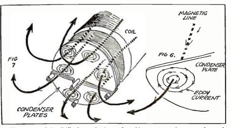
Figures 6 and 7. "A" shows the losses by eddy currents when a condenser is mounted on the end of a coil. The lines of force as indicated in Figure B show the eddy current set up when the line cuts through the plate, which wastes power.
