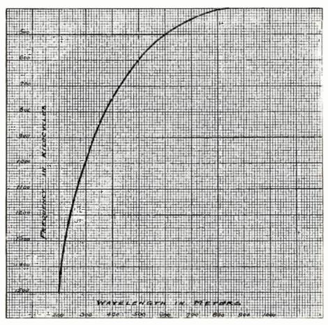
The chart above shows the relation of wave lengths to kilocycles. Notice especially how steep the curve bearing this relationship becomes as it increases in frequency and decreases in wave length.
