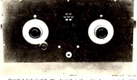
Doesn't it look simple? The rheostat's inside and is always set at the right made with about 500 value. The tube lights when the phone plug is pushed in. The left hand condenser turns of the No. 30 has a vernier control and accomplishes the tuning.
