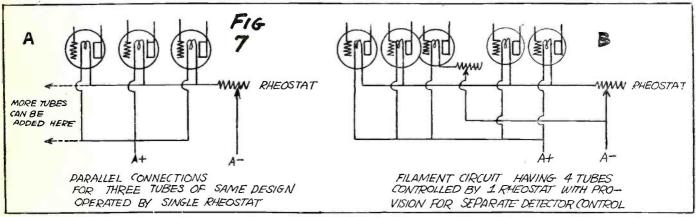
The filament circuits of several vacuum tubes may be controlled simultaneously with a single rheostat as shown on the wiring diagram above. This type of filament control is especially useful in multitube sets such as the super-heterodyne.
