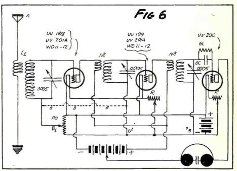
It is often necessary to connect the grid return of the second stage of RF to the potentiometer arm as shown, but should be avoided if possible. With a straight negative bias on the grid of the second RF tube, the circuit gives the greatest amplification.
