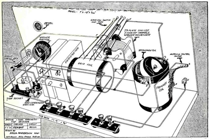
An isometeric projection of the selective receiver described by Mr. Pearne in the accompanying article. This sketch is schematically diagram:d in Figure 2, and may be used as a wiring plan if Figure 2 puzzles. The variometer is set back slightly so the grid coil will clear the condenser.
