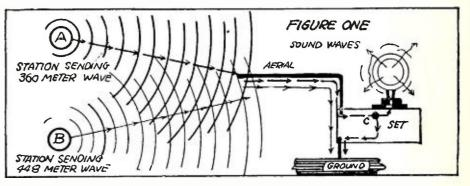
When the set as shown is tuned to Station  $\Lambda$ , the signals from that station enter the detector C and are changed to sound waves. Waves from Station B pass through the set unchanged, and go off to the ground without being converted into sound, because the set is not in resonance with that frequency.
