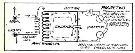
The secondary or oscillatory circuit is the part of the set which accomplishes the action of selecting the desired stations. The impulse or wave is transferred to the main tuning coil by induction and surges back and forth as indicated in the circuit shown in black. The current of a pulsating direct nature is converted by the phones to mechanical enegy.
