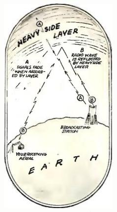
It is supposed that a "Heavy-side layer" as illustrated in the diagram above is responsible for the fading of signals, as well as their propagation along the surface of the earth. When this layer absorbs signals, we have fading.
