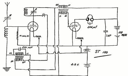
Reflex Circuits seem to be the pet hobby of the English fans, as shown in these diagrams submitted by a British broadzast listener. To the left is a one tube regenerative circuit which embodies some form of special connections for reflexing the AF on to the grid circuit Above, a two tube reflex circuit of the tuned impedance variety which uses a crystal detector. Notice the prevailing use of conductive coupling to the antenna.
