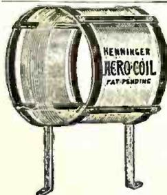
Test No. 40. HENNINGER AERO-COIL. Manufactured by the Henninger Radio Manufacturing Company, 1772 Wilson Ave., Chicago, Ill. These air-core transformers were tested in our laboratories and found to be very efficient. No. 22 D. C. C. wire is used in winding both the primary and the secondary. This reduces the high frequency resistance to a minimum. Exactly the correct air spacing between turns. Tested and approved by RADIO AGE Institute.
