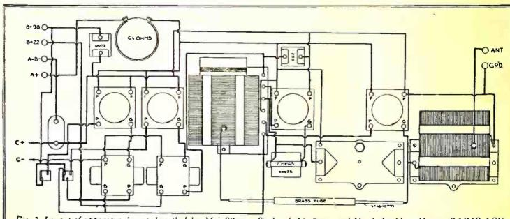
Fig. 3. Layout of apparatus in set described by Mr. Silver. Study of this figure and No. 1 should enable any RADIO AGE reader to make such a set.
