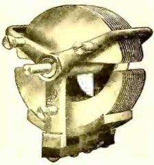
Minimum of metal in the field and frame of high resistance material reduces eddy current losses. Monoblock mounting Monoblock mounting with plates cast into block reduces series resistance and insures perfect contact with all plates. The use of only one strip of insulation answers the function of two and four pieces and reduces leakage losses proportionately. Adjustable ball bearing insures smooth rotation and constant capacity calibration.
