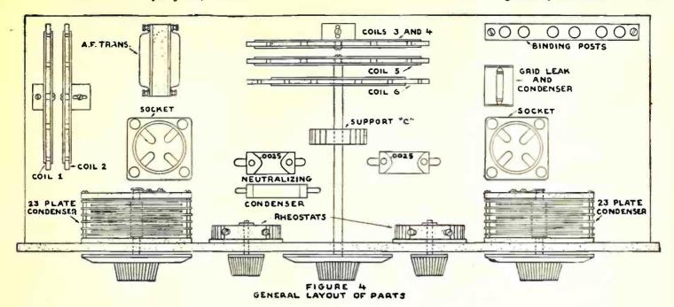
In building any kind of a set which employs radio frequency amplification, the one essential feature is to provide some way to overcome the oscillations of the radio frequency amplifier. This type of a mplification is absolutely necessary if the best results are to be
