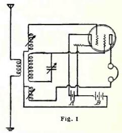
A simple hookup of the regenerative type, where the full efficiency of the double grid tube is utilized. As low as 6 volts for the "B" battery will not cut the volume of the reception appreciably in this hookup.
