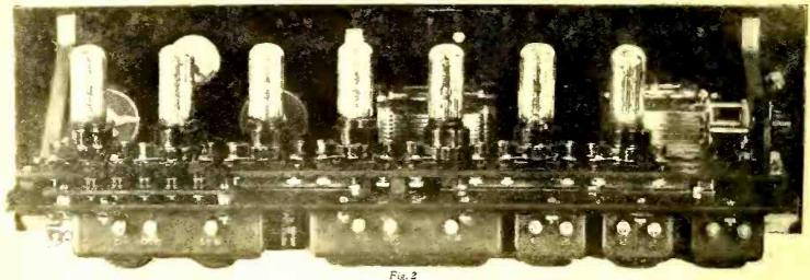
Rear view of Mr. Hopkins' receiver, showing the assembly of the sub-panel, including the transformers, which are so arranged as to conserve the maximum amount of space and make the set truly portable as well as compact.
