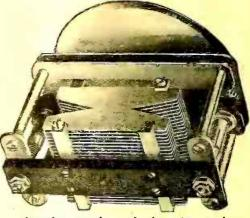
Angular cutting of the plates gives which distributes the stations evenly over the dial. This feature not only simplifies tuning, but adapts the condenser for use in wave meter and standard circuits. It also makes it possible to locate any station on the dial after once having located any station of given wavelength.
