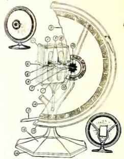
Parts in the Crosley Musicone Cone diaphragm Set screw Magnet frame 10. Armature coils Base
