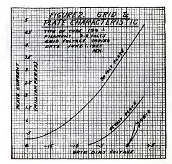
Figs. 1 and 2. Fig. 1 shows the typical curve of plate current voltage, while Fig. 2 shows the typical curves of grid and plate characteristics, the result of tests described in the accompanying article.
