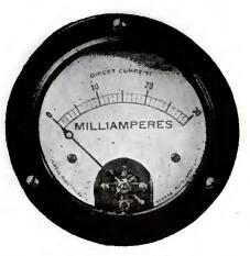
The milliameter shown above shows the plate current characteristic in milliamperes.
