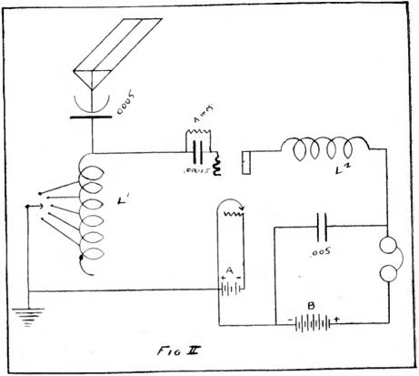
This is the single circuit Armstrong. L 2 is inductively coupled to L 1 for feedback purposes, and its relationship is variable. The inductance change in L 1 is by means of tops and the condenser in the antenna circuit. Good for results but hard on your neighbor if you let your tube oscillate
