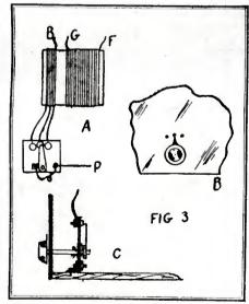
Fig. 3—Details of a variable coupler. Primary and secondary are fairly well separated, to avoid capacitative coupling. A sub-panel tap switch permits the use of any desired number of turns in the primary. White dots on the panel show where the lever is to be set.
