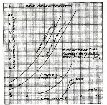
Fig. 1. A typical grid characteristic chart for 199 type (3 volt) tubes with plate voltages of 45-80 and 90 volts.
