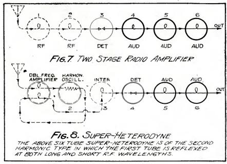
Figs. 7-8. Six Tube Circuits. Two Stages of Radio With Resistance Coupling (7), Super-heterodyne (8).
