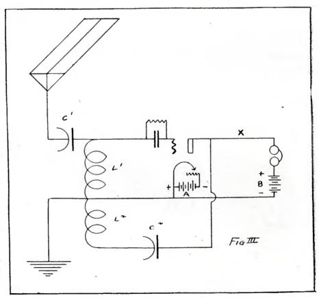
Another popular type of receiver in which regenerative control is by a variable capacity in series with an inductance paralleling the plate and filament. Known years ago as the Weagant circuit, later popularized by Reinartz and others. Better build it loose coupled for the sake of the neighbors, unless you happen to live out in the exact geographical center of the Gobi desert
