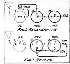
Three Tube Circuits Com-Dotted Line Represents Figs. 1-2. monly Used. Radio Frequency and Solid Line is Audio Frequency.
