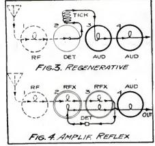
Figs. 3-4. Four Tube circuits, Regenerative, With One Radio Stage (3) and Reflex Four Tube (4)
