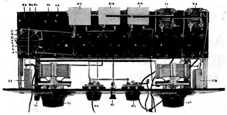
Interior view of the super-autodyne. The instrument designations will be found in the text. The sockets, from left to right, are: V1, autodyne; V2, 1st R. F.; V3, 2nd R. F.; V4, 2nd Det.; V5, 1st A. F.; V6, 2nd A. F.; Socket shelves may also be procured for UV199 or C299 tubes.
