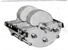
No. 71, CONTINENTAL 2-GANG CON-Test No. 71, CONTINENTAL 2-GANG CON-DENSER. Submitted by Gardner and Hepburn, Inc., 2100 Washington Ave., Philadelphia, Pa. Con-sists of a two gang variable condenser, well made and suitable where tuning of two inductances simul-taneously is desired. Or it can be used with the two halves in series to decrease the capacity of the con-denser. Tested and approved by RADIO AGE In-
