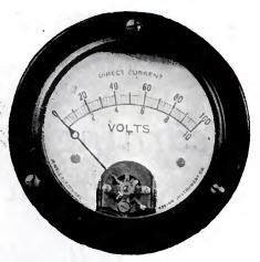
The 0-10, 0-100 scale voltmeter, which shows the filament voltage and plate voltage, respectively.
