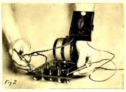
Fig. 2. A neat and efficient means of testing for breaks in wiring of sets, which can be applied to almost any use in determining the continuity of wiring in coils, transformers, phones, and other apparatus.
