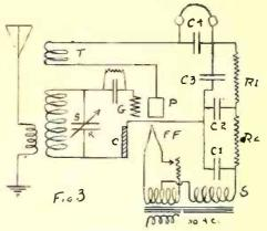
Fig. 3. This is a typical one tube regenerative circuit with the A. C. tube arranged so it also delivers B battery current in addition to the A current.
