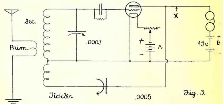
Fig. 3—Weagant-Reinartz circuit for the space wound coil and parts as used in the usual three-circuit tuner. This method of regeneration control doesn't interfere with the setting of the tuning dial. Try it.
