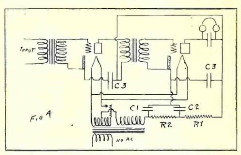
Fig. 4. The alternating current tube adapted to the two stage amplifier in which the B battery potential is also produced by the A. C. tube.
