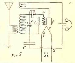
Fig. 5. Now we are using 110 volts on the filament instead of a lower voltage. Also we are supplying the plate potential through the rectifying properties of the same tube.
