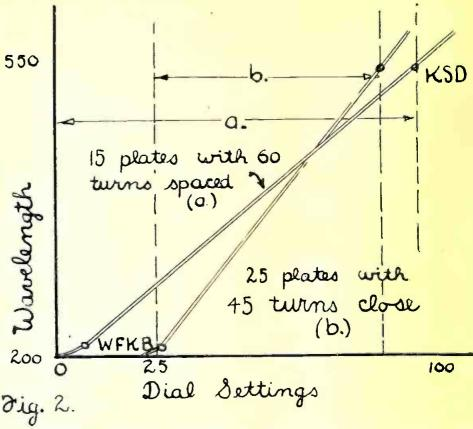
Fig. 2—Comparative luning curves showing the advantage gained by using a space wound coil and a smaller condenser. The 15-plate condenser was made by removing five of the rotor plates from the 25 plate instrument, the corresponding 5 fixed plates thus not being used.
