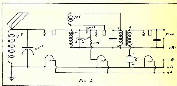
This is the general type of tuned radio, detector and one stage of audio amplification in use in the British Isles. It is sent in by
