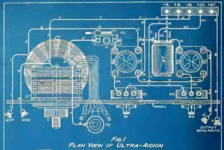
IN ORDER TO SHOW THE OUTPUT CONNECTIONS FOR EITHER JACKS OR BINDING POSTS AS MAY BE DE-SIRED, WE SHOW POSTS IN FIG. I AND JACK IN FIG. 2.
