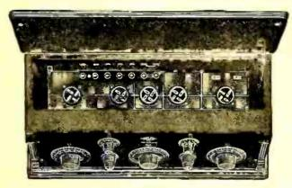
N TESTING the Melco Supreme receiver we experienced a few new things, both in circuit design and use of radio apparatus. The Melco Supreme receiver is a tuned radio-frequency receiver using five tubes, and follows the usual design in such a circuit. The differences that exist are not in any way radical but they represent refine-wents in parts of the circuit that are im-
