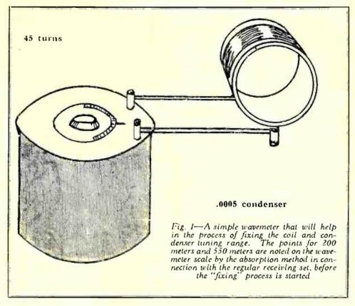
and that fewer turns of wire will be needed to place the lowest wavelength at the desired point—200 meters for broadcast reception. The effect of the tuning condenser is thus decreased; that is, a larger condenser is necessary to cover the broadcast band.
