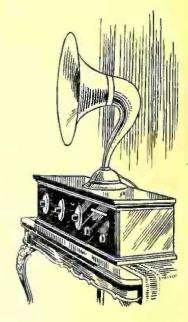
Correcting the Erroneous Impression that All the Energy Comes from the Transmitter; Power Creating Sounds in Home Due to 'B' Voltage
