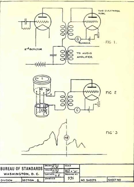
amplifier or detector tube. Since changes in crystal sensitivity, due probably to contact variations, sometimes produce records very similar to fading curves, this method is not altogether dependable.
