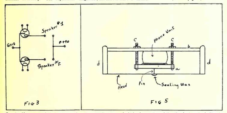
Fig. 3— Using two loud speakers to cover the entire musical range, one for higher frequencies and the other for low; the double tube connection allows a separate tube for each speaker. Fig. 5—Details of the mandolin low-note loud speaker.
