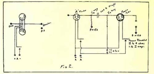
Fig. 2—To prevent overlooding of the lost oudio tube, o heavy power tube moy be employed, or as an alternotive neorly os good, two tubes moy be operated in porallel.
