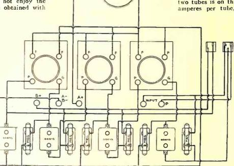
Figure 2. Wiring diagram for distortionless audio amplifier. As all parts have been illustrated pictorially, rather than in symbols, this diagram is very easy to follow, even by the inexperienced set builder.
