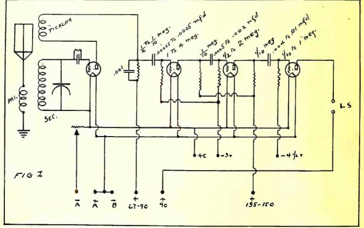
Fig. 1—Circuit-for o three-stoge resistonce-coupled oudio omplifier together with the detector connections, showing how three different plote voltoges ore required.
