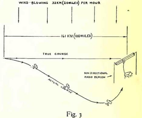
EFFECT OF WIND DRIFT ON AIRPLANE, SHOWING COURSE TAKEN BY AIRPLANE WHEN FLYING AT IG KM (IOO MILES) PER HOUR AND NAVIGATING BY MEANS OF DIRECTION FINDER BEARINGS ONLY.
