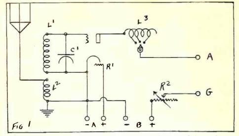
Fig. 1. In this r. f. unit, to go ahead of a regular set, submitted by Robert A. Del ries, 114 8th Ave., New York City, N. Y., readers may find a solution to their worries about the lack of signals. The variable resistance in series with a tapped plate coil allows the control of the plate potential and helps prevent undue regenerative effects in the first tube. The description is given elsewhere in this department.
