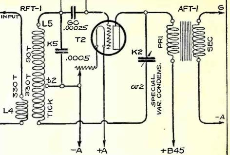
regenerative similar to the first stage, except for the addition of the grid condenser and leak. With the two circuits coupled together, we have a cascade regenerative circuit with its output connected to the first audio frequency transformer (AFT-1). Following the detector are three audio stages of the usual type for increasing the audio volume of the detector.
