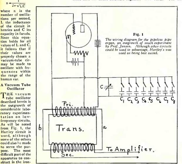
C2, C3, etc. were made out of an old high-voltage paper condenser. Trials with small laboratory units showed that the value of C1 should be about .01 Mfd. to give a pitch of C - 256 vibrations per second. A paper condenser of that magnitude was connected in and the pitch tested against a tuning fork. Approximate adjustment was made by trimming the tinfoil between layers of paper, and final tuning to the exact note was obtained by the use of the variable condenser.
