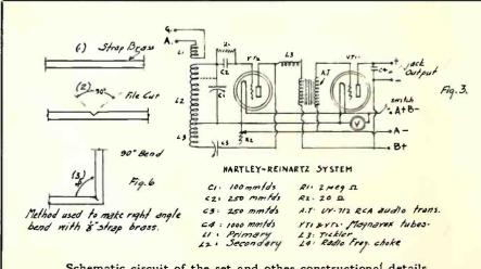
Schematic circuit of the set and other constructional details
