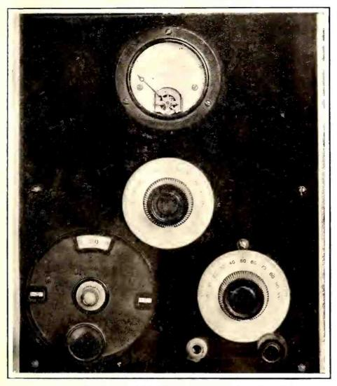
Front panel view of the short wave receiver
