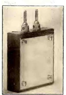
Quartz plate holder for piezo oscillator assembled
