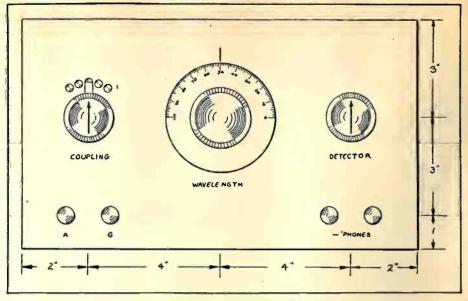
Fig. 2. Simple panel layout for the crystal set
