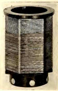
Improvement has been noted in the winding of the Silver-Marshall interchangeable plug-in coils. Instead of the winding being of silk covered wire wound close together (for the longer waves) the forms are now supplied with threaded supporting columns on the coil and the winding is done with enamel wire, each turn fitting into its groove. Thus the capacity effect between adjacent turns is reduced. The coils are available from 18 to 550 meters and fit the S-M universal coil socket.
