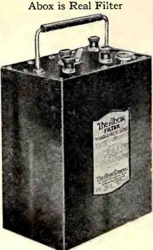
**BATTERY** elimination has arrived with a bang if recent tests conducted in the Radio Age laboratory are any criterion. The new device, as developed by E. F. Andrews (of Deresnadyne fame) and Laurens Hammond, both of Chicago, comprises a filter and a choke, the former being the work of Mr. Andrews on which patents are now pending.
