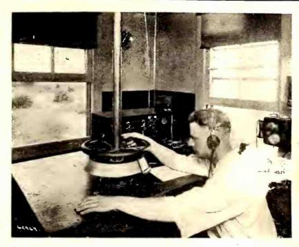
Radio operator at compass station obtaining bearings on a vessel. America's merchant marine has come to depend upon this service as a means of saving time, money and life
