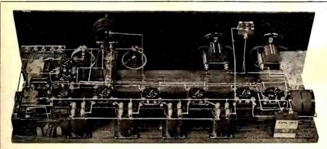
Rear view of the completed receiver as adapted for storage battery tube use. Tube sockets are mounted on an elevated strip so the long wave transformer leads to sockets will be but an inch in length
