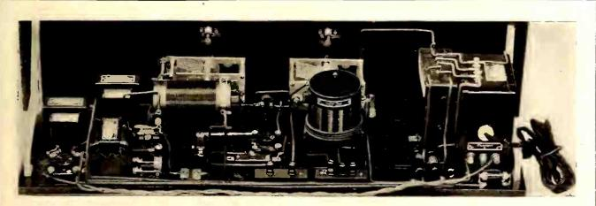
Rear view of the completed Browning-Drake power operated receiver, parts for which are shown in list on the opposite page
