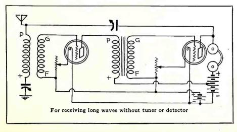
the amplifier tube. The device is similar to a rheostat but has terminals at both ends and a sliding contact in the middle which is connected with the lower end of the secondary coil of the first transformer, or to the ground.
