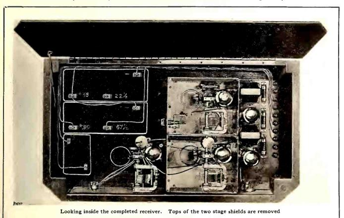
No shield is necessary on the first radio frequency stage although the receiver is designed so that a shield can also be used for this stage if desired.
