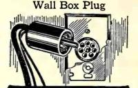
OWARD B. JONES of Chi-LL cago, manufacturer of the Jones Multi-Plug line for battery connections, announces a new type W. B. (Wall Box) Multi-Plug, consisting of the standard seven contact socket mounted on a switch box cover and the regular plug and cable.
