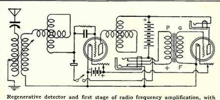
Regenerative detector and first stage of radio frequency amplification, with crystal detector for use when tubes are cut out
