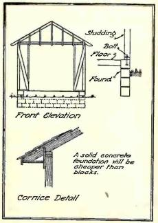
After the sills have been bolted down the studding, spaced two feet on center, are erected as shown, excepting the space for the front and side doors. The corner posts should be of doubled two by four inch pieces, nailed together. Note that in the front, bracing is accomplished by one by four inch boards, mortised into the studding flush with the surface. The dotted lines of the side elevation show how additional bracing can be used if deemed necessary.
