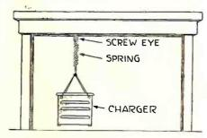
Secure a strong wire to each of the four corners of the charger case. These can be attached by running them through the ventilating holes. All four wires are joined and fastened to a door spring. The charger is then hung from a large screw eye under the table, it need not clear the floor by more than an inch or so. See illustration.—J. C. Heberger
