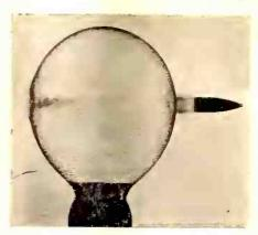
THE BULLET AND THE BUBBLE phtogr aph made in the sound laboratory of the U. S. Bureau of Standards by means of an electric spark, by Philip P. Quayle, showing a soap bubble through which has been fired a rifle bullet. The bullet has passed out of the bubble, but it still stands, with a hole in each side. The lines extending from the front of the bullet are sound waves
