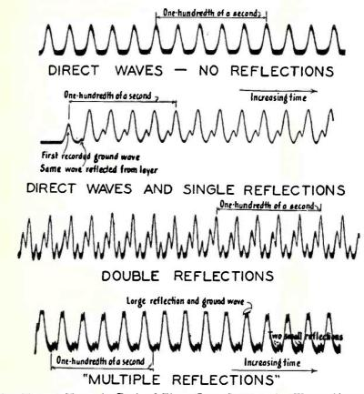
The Highest Hump in Each of These Cases Is Made by Waves Along the Shortest Path; the Smaller Humps and some of the Irregularities Are Caused by Reflections
