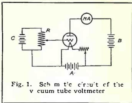
Fig. 1. Schematic circuit of the vacuum tube voltmeter
