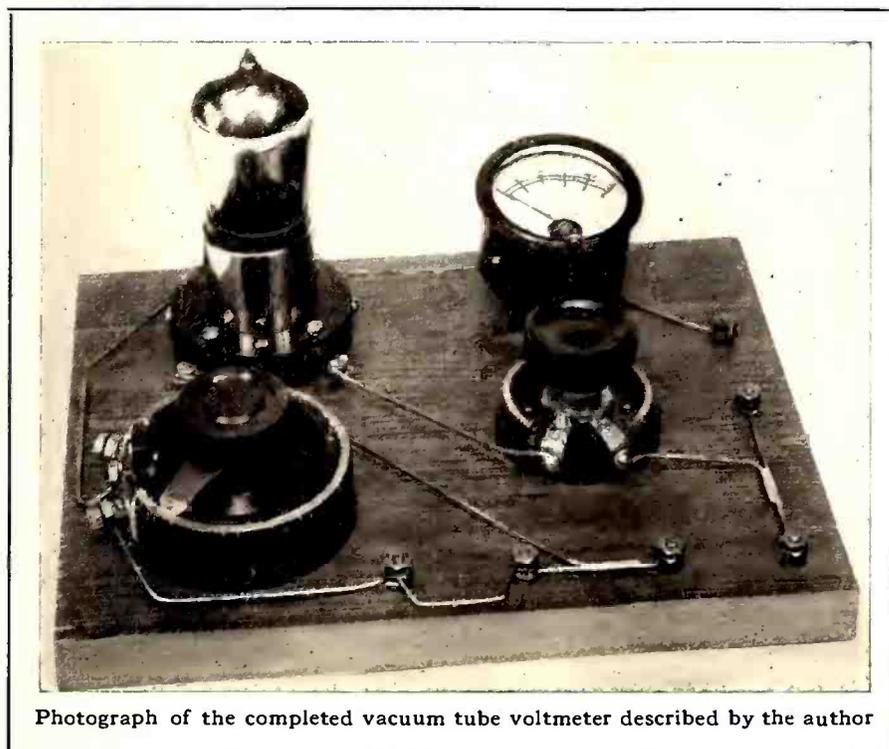
Photograph of the completed vacuum tube voltmeter described by the author
