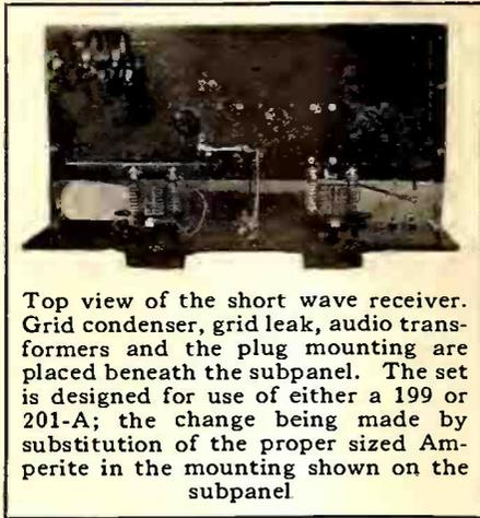
Top view of the short wave receiver. Grid condenser, grid leak, audio transformers and the plug mounting are placed beneath the subpanel. The set is designed for use of either a 199 or 201-A; the change being made by substitution of the proper sized Ampelite in the mounting shown on the subpanel.
