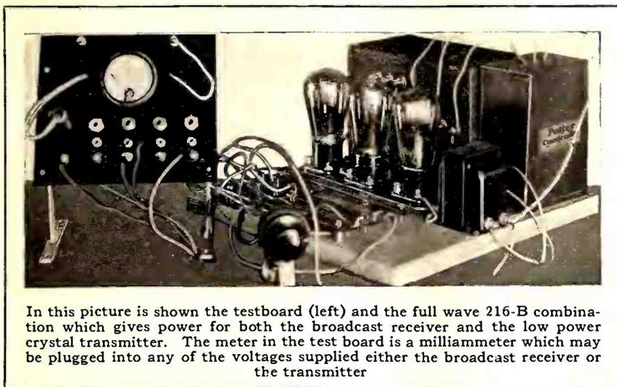
In this picture is shown the testboard (left) and the full wave 216-B combination which gives power for both the broadcast receiver and the low power crystal transmitter. The meter in the test board is a milliammeter which may be plugged into any of the voltages supplied either the broadcast receiver or the transmitter
