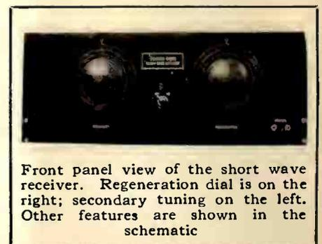
Front panel view of the short wave receiver. Regeneration dial is on the right; secondary tuning on the left. Other features are shown in the schematic
