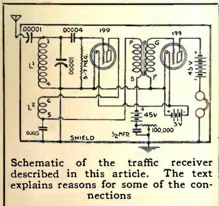
Schematic of the traffic receiver described in this article. The text explains reasons for some of the connections
