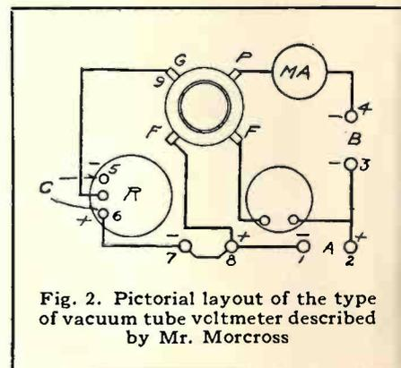
Fig. 2. Pictorial layout of the type of vacuum tube voltmeter described by Mr. Morcross
