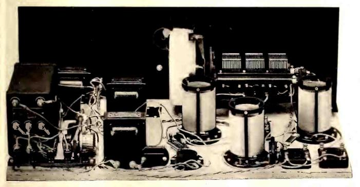
Rear View of A. C. Operated Receiver Showing Placement of Parts and Associated Wiring. The Set is Wired with Flexible Rubber Covered Wire, Simplifying Wiring and Construction. The 171 Bias Resistor and By-pass Condensor are Hidden from View Behind the Out-put Transformer.
