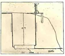
Several coolers of this type have been installed at the Fairlawn golf course near Akron, Ohio. from the surface sprinkling system often reaches a temperature near the boiling point, but after being passed through the tank it emerges from the fountain at about fifty degrees Fahrenheit.
