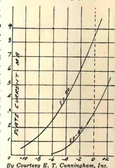
Fig. 4. Plate current grid voltage curve
