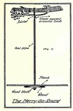
merry-go-round that is really different. Fasten a short piece of chain to a limb and attach a swivel to it, preferably with a ring. Attach a longer chain to this and run it through a gas pipe. Fit a large iron wheel with a plank on top onto the lower end of the pipe, setting it fast with a set screw. The lower end of the chain is kept from slipping up the pipe by tying or otherwise securing it to a block of wood or piece of iron.
