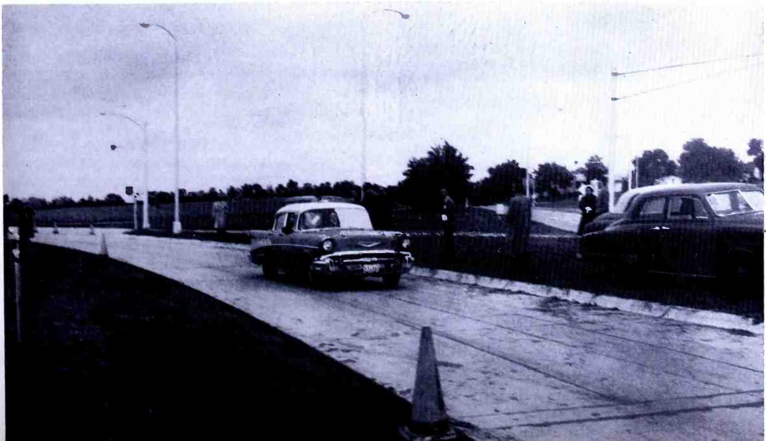
Cars with radio receivers run tests on highway equipped with buried detector circuits at Lincoln, Nebraska. RCA scientists are continuing developmental work on system.
