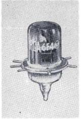
The acorn was the first successful tube for the reception and transmission of UHF signals.
