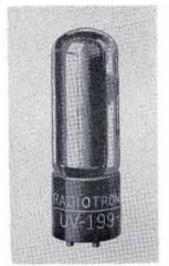
Portable receivers were popularized when RCA developed the battery operated 199 tube. Then radio sets were carried out of the homes.
