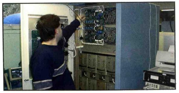
Fine tuning: A technologist adjusts the IPM compensation for optimum AM IBOC performance on the XL 12 model at Nautel's lab in Halifax, Nova Scotia.
