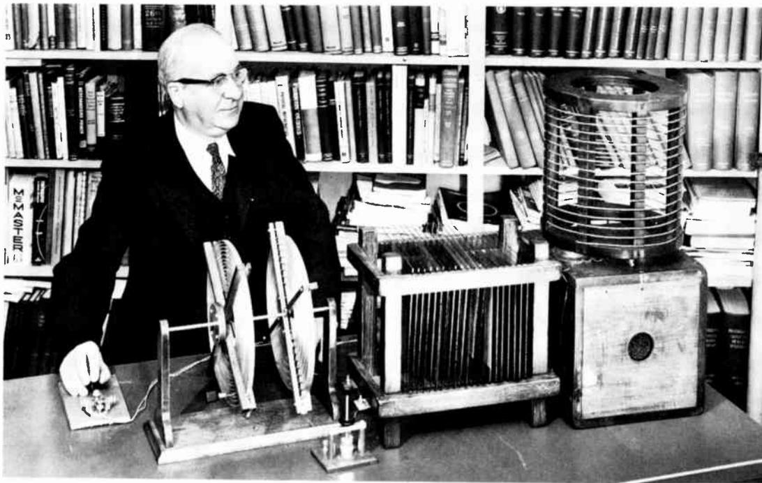
The fifty-year old spark gap of this wireless transmitter, pounds out the introductory message of the Golden Jubilee LP Record. Harry Houck, owner and builder of the equipment, is the operator.
