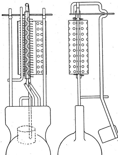
Fig. 8. Construction of perfected quick-heater audion.
