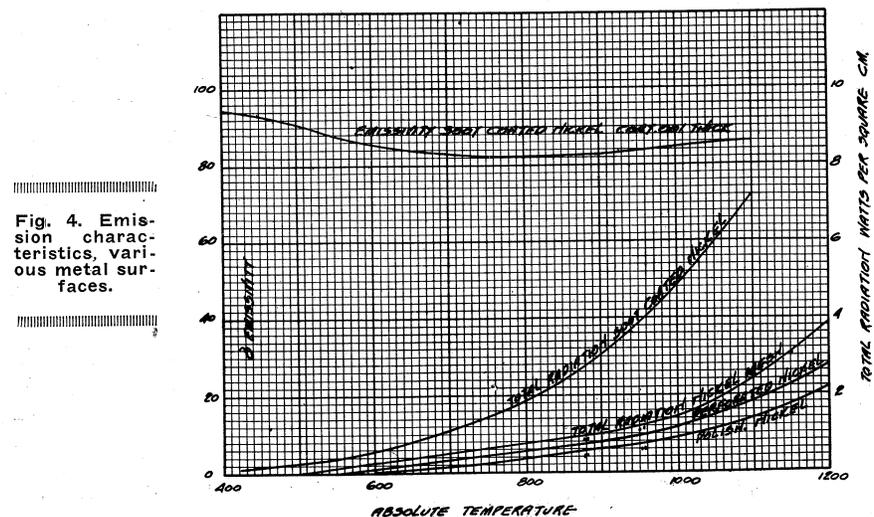
Fig. 4. Emission characteristics, various metal surfaces.
