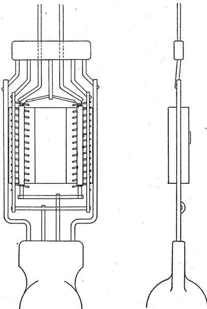
Fig. 1. Early 5-volt heater tube assembly.
