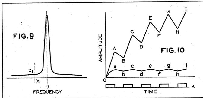
Fig. 9. Typical resonance curve of highly selective circuit.
