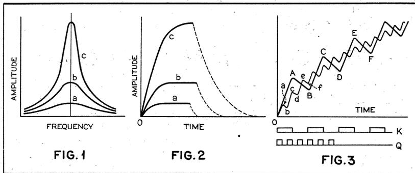
Figs. 1, 2 and 3. Damping, amplitude and response curves, respectively.
