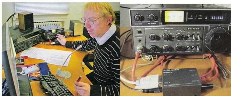
Figure 12 Ray Jacob, W2RJJ, (left) operating his SSB 50 MHz amateur radio station provided with Internet-operability. The sound card interface to his transceiver (right). The VoIP (Voice over Internet protocol), and EchoLink operation, allows him to speak both to amateurs locally, radio link(s), as well as to amateur radio operators where-ever
