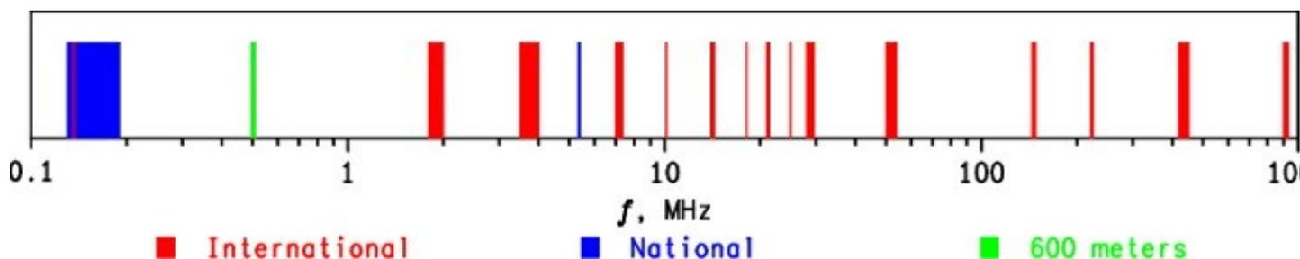
Figure 1. Amateur-radio spectrum from 100 kHz to 1 GHz.
