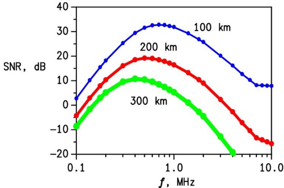
**Figure 8.** Ground-wave signal-to-noise ratio.
