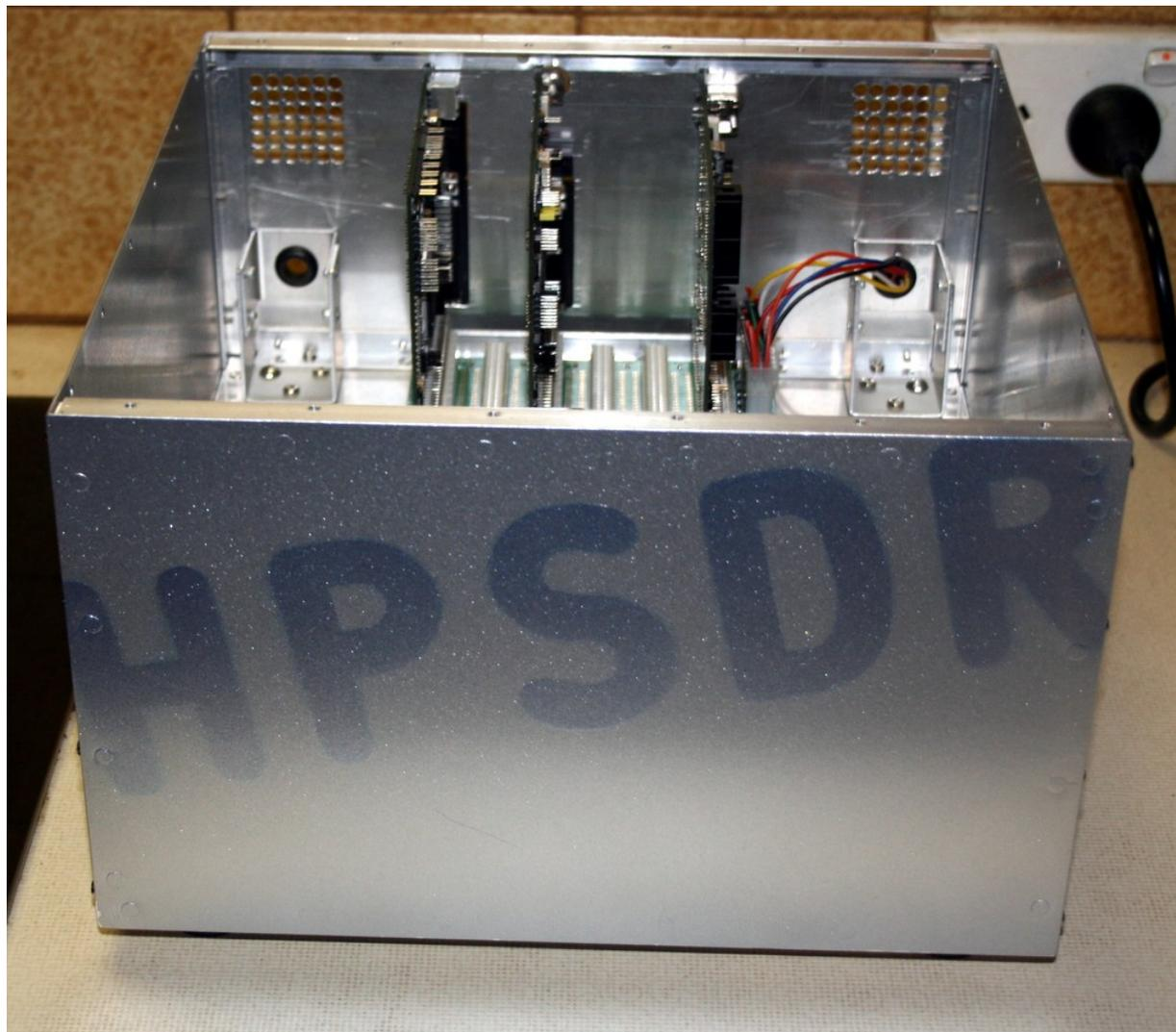
**Figure 6** VK6VZ's partly-built HPSDR transceiver in VK6CG's prototype case.
