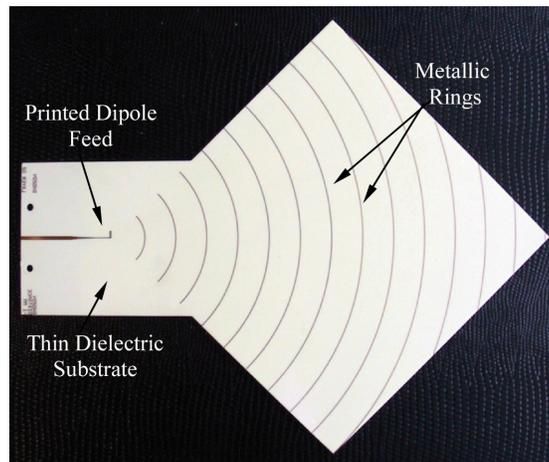
**Figure 10.** Integrated printed dipole feed and holographic-designed antenna.
