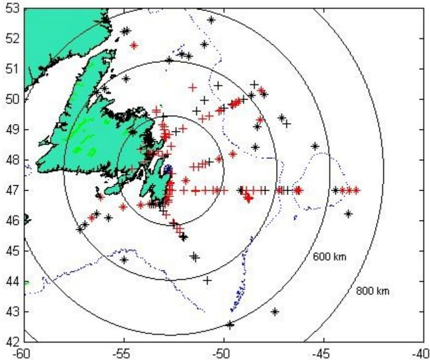
*Figure 9* Receptions of the 10 watt 187 kHz beacon. Red symbols indicate readable signals, black symbols indicate no signals heard. Note how a reception path over the ocean extends farther than those over the land.
