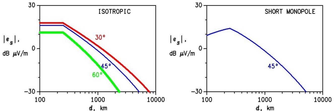
**Figure 9.** Median MF sky-wave signal strength.
