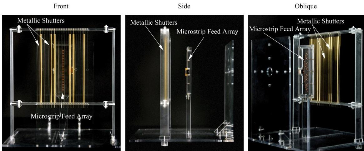
**Figure 13.** Fresnel zone plate shutter antenna with beam scanning capability.
