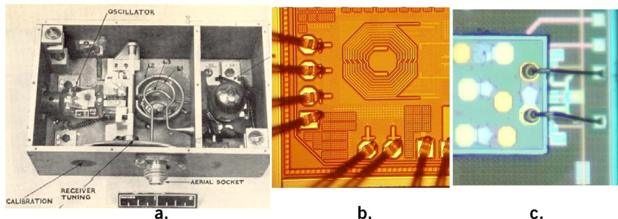
Figure 3. Evolution of RF design showing a.) Bulky vacuum-tube design using high quality passives, b.) Current RF design using on-chip passives, and c.) Our vision of future RF design using fast commodity transistors and high-quality passive devices
