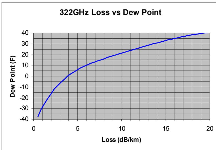
Looking forward at even higher operational frequencies, one must face the fact that atmospheric losses will even be that much greater and modern DSP receiving techniques that involve very long integration times must be considered if even the slightest value of received carrier-to-noise is to be expected.
