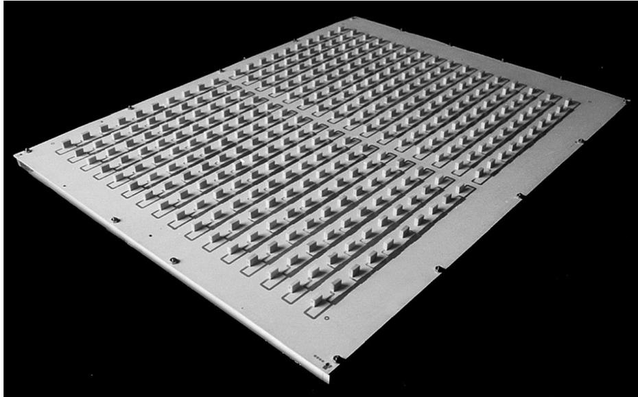
**Figure 1.** Phased array of multi-segment DRAs with electronic beam steering, designed at 8 GHz.
