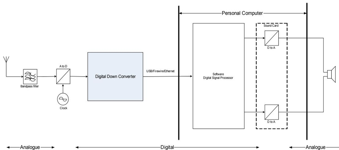
**Figure 4 Block diagram of a DDC-based receiver.**
