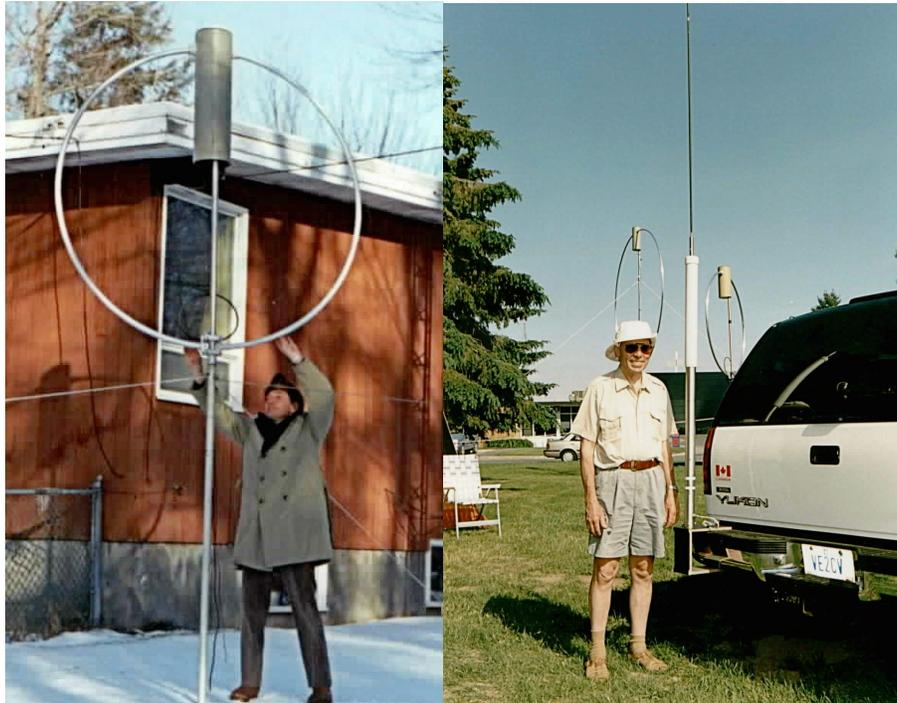
**Figure 5** Author Belrose experimenting with an AMA 1.7 m diameter loop, on the left, and, on the right, two compact loop antennas and a vehicular mounted HF whip antenna, a tunable all bands antenna (TABAs), in use during a simulated emergency communications exercise.
