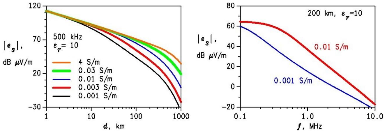
**Figure 7.** Amplitude of the ground-wave signal.
