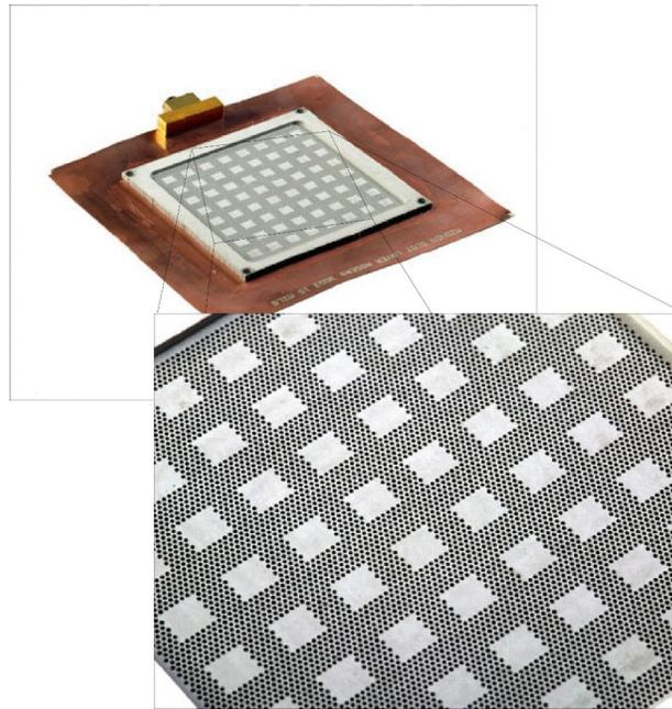
**Figure 3.** Array of perforated DRAs, designed at 24 GHz.
