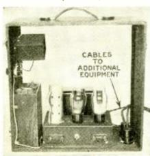
Close up of the Lafayette Dual Speaker Portable Amplifier. Along the left side are (top to bottom) mike coupling transformer, gain control, and mike batteries.
