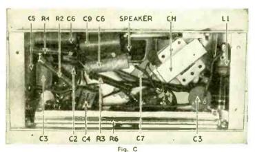
Under-chassis view illustrating the location of detail parts.
