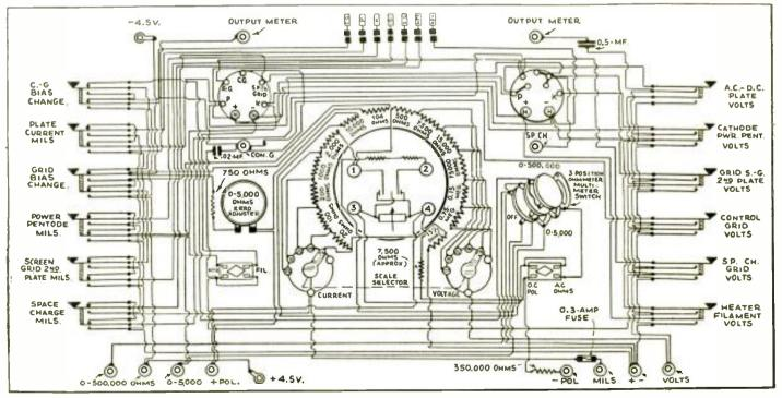
Complete schematic circuit of the Supreme model 90 set analyzer "revamped" to take care of the latest circuits.
