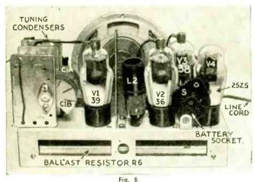
Rear view of the receiver showing the location of parts.
