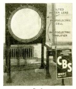
Photograph of the receiving lens and the photoelectric cell used in the experiments.
