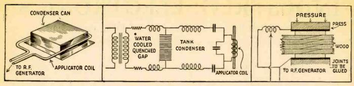
Fig. 4-H.F. heat solders condenser cans. Fig. 5-A quenched-gap type of H.F. heater. Fig. 6-A set-up for H.F. gluing of plywood.
