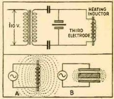
Fig. 1—This experimental unit heats nails.
