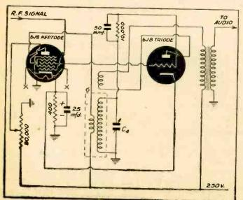
Left—Part of the circuit of "Mystery" Martin's 4-tube receiver, showing action of the 6J8. Below — How the neon-oscillator may be adapted to work from the line or power pack.
