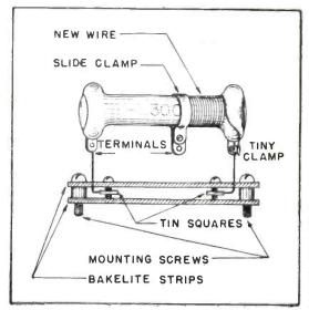
Wind over the same resistor the amount of wire required to satisfy your needs, then put over the new terminal a previously fixed slide clamp from a discarded resistor, and ... Oh, yes! A mounting. Solder two little squares of tin or brass sheet to the wire points of the resistor. Get two strips of bakelite or other similar material. Make two slots in one of the strips to receive squares and wire, bend wires properly. Drill two holes on strips of bakelite so you can mount on chassis.
