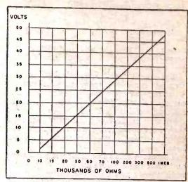
Fig. 3—Specimen chart of the ohmmeter scale.
