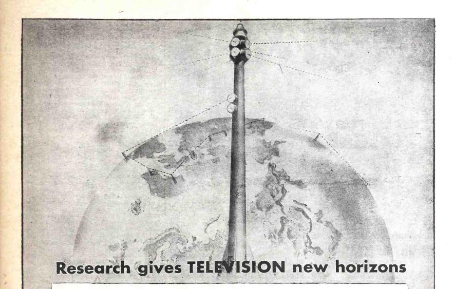
• TELEVISION RAYS—like human sight—do not "bend" far beyond the curvature of the earth. They travel in a straight line to the horizon—and from the horizon off into space. In preparing television as a service to the public, research has sought ways to extend television's program service by radio relaying from city to city.
