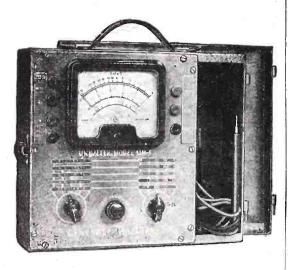
• Completely portable all-around utility instrument, ideally suited for reliable service work. Large meter calibrated to reduce the error possibility in readings makes the G-E unimeter a popular one with servicemen.
