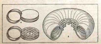
Fig. 1, left—Evolution of a resonant-cavity circuit from the coil-condenser combination may be traced with the help of this diagram. Right — Cut-away photo of a typical Klystron.
