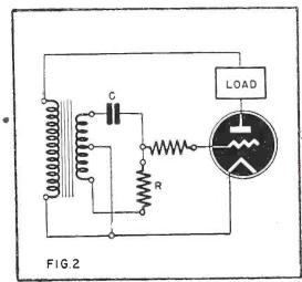
Fig. 2—By correctly proportioning C and R the desired shift of phase may be obtained.
