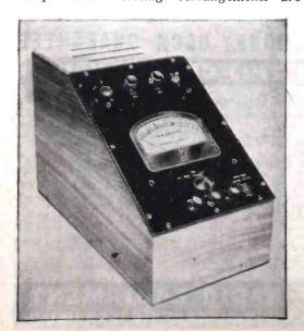
provided for the rapid charging of condensers under test. An external battery voltage supply may be used where voltages other than the self-contained 200-volt supply, are desired. The instrument may be satisfactorily operated with external voltages up to 1000.
