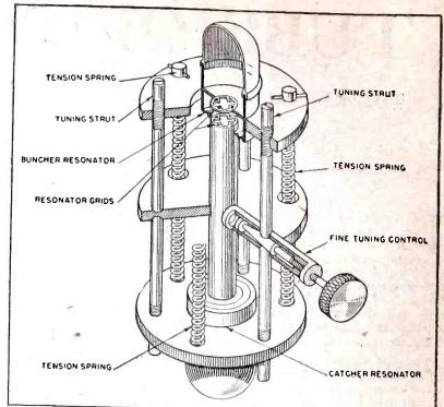
Fig. 2, left—Schematic view of the Klystron. Fig. 3, top—How the tube is tuned. Coarse adjustments are made with the three large struts, fine tuning by varying one against the other two.
