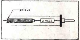
Fig. 2—Construction detail of the test probe.
