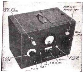
The voltmeter is housed in a semi-portable cabinet. The various controls are indicated as an aid to the constructor.
