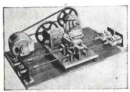
On one-half cycle, the wiper travels from minimum to maximum resistance and reverses in the next half cycle, simulating manual operations at a continuous high rate of speed which is, in itself, more abusive than normal operations would be. New models and spot checks are run as many as 200 hours at rates stipulated in American Standards Association specifications. Upon examination—and the parts are completely disassembled and examined they have required no repair or adjustment.
