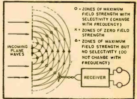
Incoming waves strike a metal baffle containing slits. Their width may be equal to the wave length of the signals and their spacing several times greater. As a result of spreading, cylindrical waves are formed beyond the baffle, resulting in weakening and strengthening of energy at different points, as shown. Positions of maximum and minimum strength will vary with the frequency.
