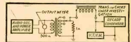
Fig. 3—A Comparator for audio frequencies.
