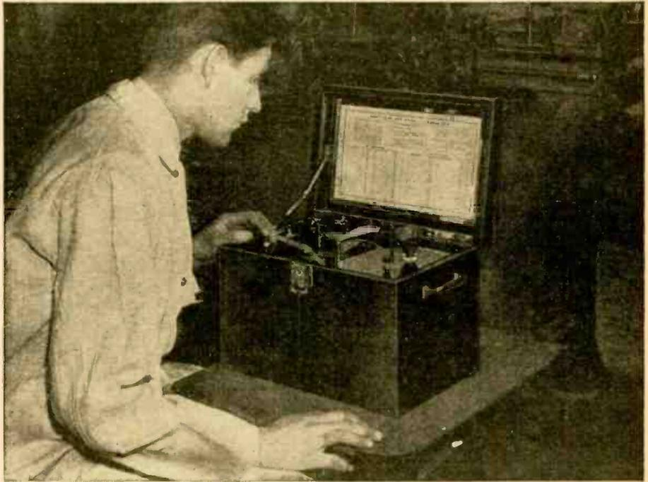
TIME-SAVING carbon content analyses of steel samples—from molten metal to report—take only five minutes with the portable, battery-powered Carbanalyzer, produced by the Fisher Scientific Company. Leading steel firms employing open hearth or electric furnaces quickly make carbon determinations of each batch, achieving close control of quality.
