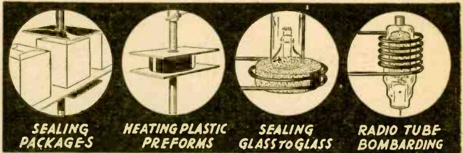
THE art of Radiothermics is divided into two branches:—*Induction and Capacitative Heating.*
