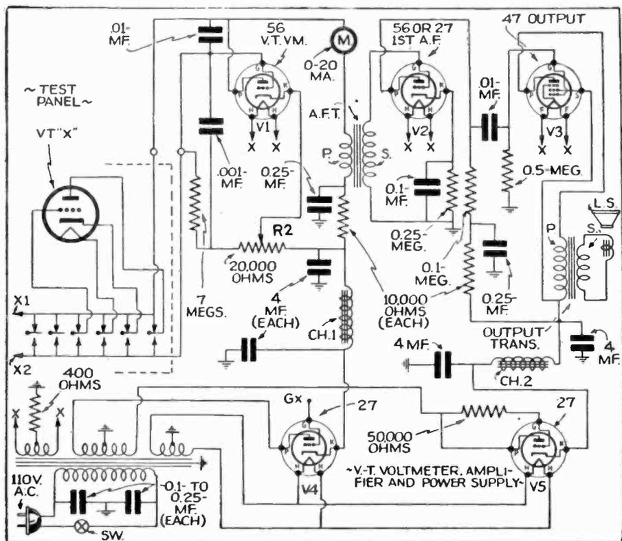
Fig. 1. Circuit of infinite-resistance tube checker.
