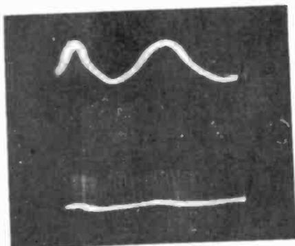
Fig. 10. Signal applied to one input while the other is open leaving input No. 2 ungrounded results in departure from a straight line.
