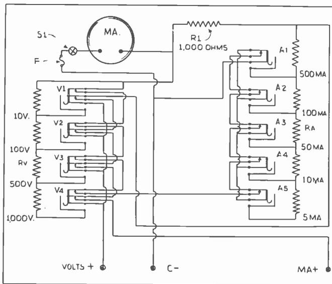
Fig. 1. Schematic diagram of the fool-proof beginners' volt-milliammeter.
