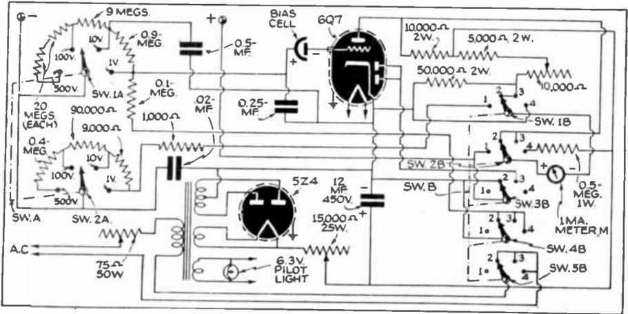
Fig. 1. Schematic diagram of the modern V.-T. voltmeter. The circuit is actually a 1-volt meter, the higher ranges being obtained by the voltage-divider resistors mounted on the range switch.
