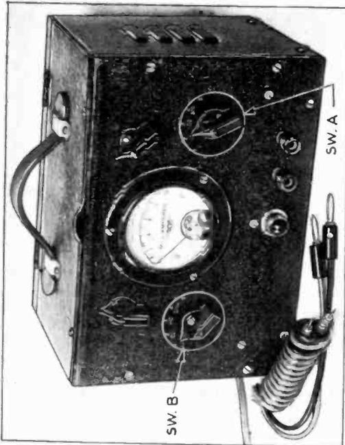
Fig. A. The V-T. voltmeter uses a 1,000 ohms/volt, 0 to 1 ma. meter.
