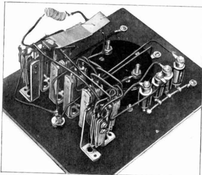
Fig. B. The inside "works" of the instrument. Two additional range jacks were subsequently added as shown in the circuit at left.
