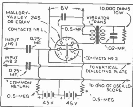
Fig. 2. Schematic circuit of the vibrating switch.
