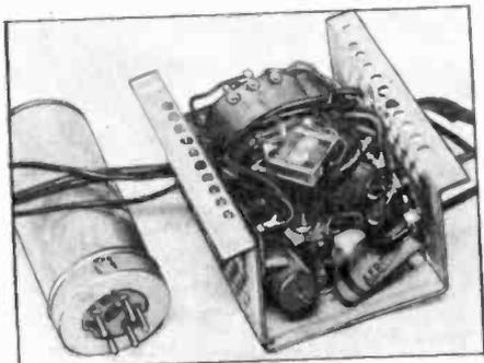
Underside view of the compact "vibrator switch" required in double-tracing your oscilloscope.
