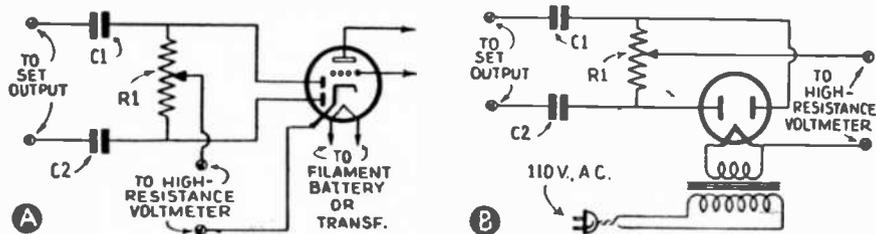
Fig. 2. A compact rectifier, to use a standard D.C. meter for testing output of radio receivers.
