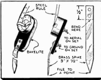
Now take a strip of brass 9 ins. long and  $\frac{1}{2}$ -in. wide. This is bent and bolted to the bakelite as shown in the sketch. A terminal is also provided. In use, the pointed end of the brass strip is pushed into the ground, which should be dampened if it is dry, and the rule extended. The aerial and ground leads are taken
