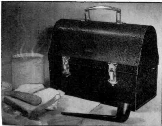
Fig. A. This humble-appearing "lunchbox" is a radio set!—complete with self-contained power supply and extensible antenna—ready to operate, at a moment's notice, and at loudspeaker volume.
