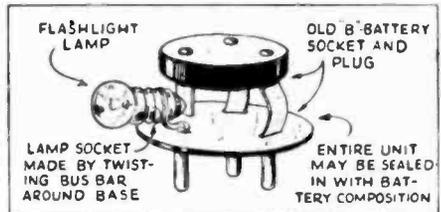
goes through the flashlight lamp. In case of a short the lamp burns out before anything can happen elsewhere. The lamp must of course have a current rating less than the total filament drain of the tubes being protected. The lamp must be bypassed by a condenser; 2 mf. ordinarily is about the right value (to prevent motorboating).
