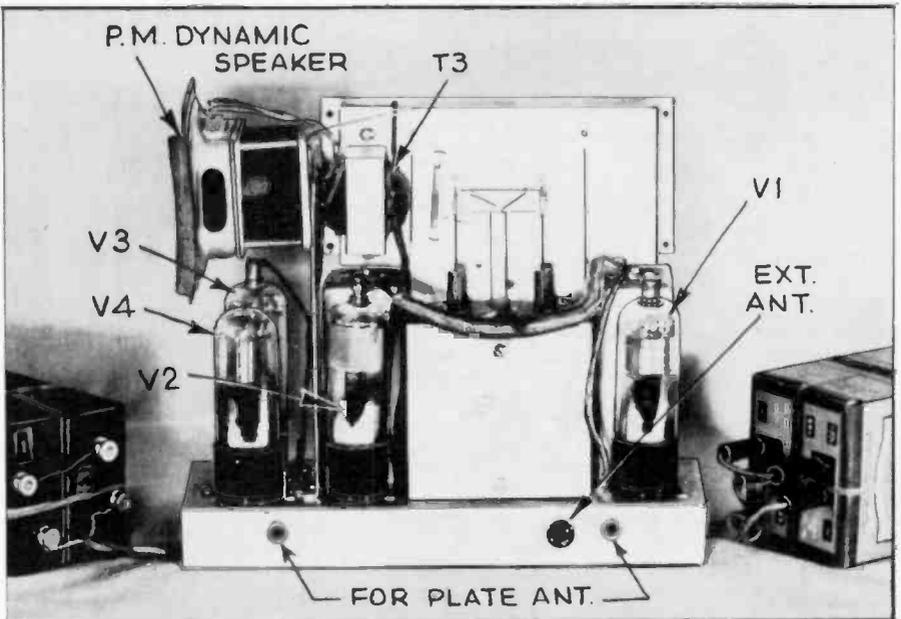
Fig. 8. Rear view of the portable showing the locations of the tubes and other components with respect to the permeability tuner. The antenna plate plugs into the 2 extreme jacks and may be used for local reception. When in the country, away from stations, use a 20-ft. length of wire plugged into the remaining jack.
