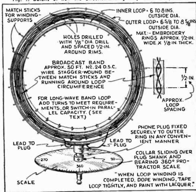
Fig. 2. Detailed specifications on the construction of the loop.
