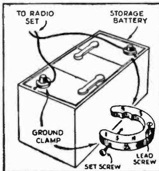
Ground clamp makes good battery terminal.
