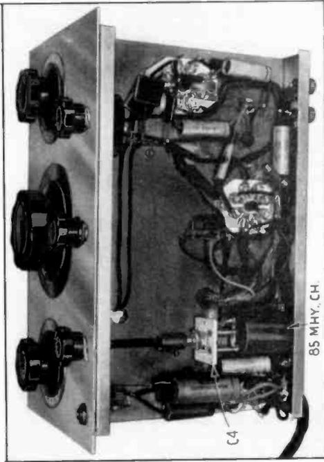
Fig. 8. Under-chassis view showing the wiring and placement of parts.
