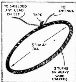
Noise-bucking pick-up coil for car radio.
