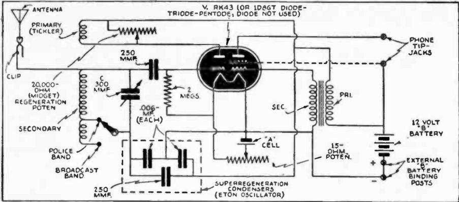
Schematic circuit of the 2-in-J "Card File" Battery Set. If tube V is a 1D8GT, connect the screen-grid as shown dotted. Condenser C is a revamped 15-plate Cardwell midget unit. Volume increases with increase of "B" voltage. Use a short aerial or a suitable condenser in series with the aerial.
