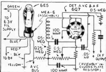
Fig. 5. Connections for the 6E5 "eye" tube, V7.
