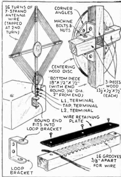
Fig. 2. Details of the collapsible loop.
