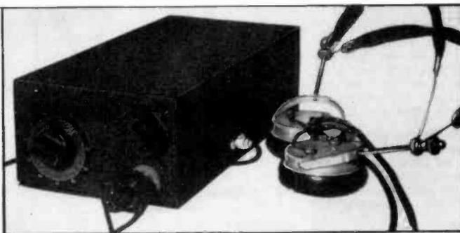
View of completed "3-in-1" Portable; antenna plugs into jack on right side. Set fits into overcoat pocket or a briefcase.
