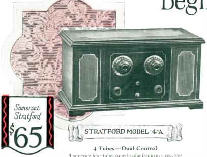
A superior four tube, tuned radio frequency receiver—two dial control—operates on storage battery or dry cells. Automatic filament control insures long life of tubes. The finest "low loss" condensers and the famous SOMERSET Calibrated Transformers are features. "B" battery space is provided in the handsome two-tone mahogany cabinet.
