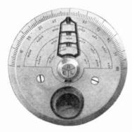
mark. All pencil-marks may be erased and the dial left like new, if it becomes necessary to revise markings, due to moving, or a station discontinuing or wavelengths changing. In addition, the Ultravernier is a single control, a further ideal simplification.
