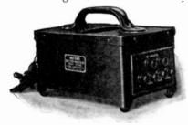
alternating current from the light lines into current of the proper magnitude and at the proper voltages and other characteristics suitable for operating the MA-20 Receiver. The Recto-Filter cannot be used with any other type of receiver than the Mu-Rad MA-20. This unit uses either one or two standard UV-201A or similar tubes.
