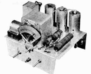
Left: A close-up of the shortwave converter chassis. The four tubes are along the back edge, the coils above and below the chassis in the right foreground. Below: the under side of the chassis, showing the other three coils grouped around the wave-changing switch.
