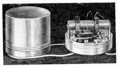
A close-up of one of the intermediate frequency transformers used in all the Pilot super-heterodyne receivers. The two coils are wound on an impregnated wooden form. The small balancing condensers are just underneath.
