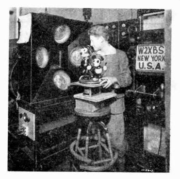
Above: the television transmitter constructed in 1928 for station WRNY, New York, by the Pilot Electric Mfg. Co., now the Pilot Radio & Tube Corporation. Left: the television transmitter used experimentally during 1931 by station W2XBS, of the National Broadcasting Company, New York. Note that the 1928 transmitter is almost identical in construction with the 1931 outfit. Both use arc lights. scanning discs and large photo-electric cells in an upright frame.
