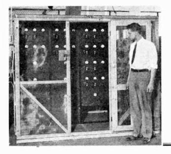
Left, Fig. 5: The signal generating booth, containing half a dosen miniature transmitters, all crystal-controlled. These are connected by shielded cables to the test cages pictured in Fig. 6. This complicated apparatus was designed and constructed by J. L. Montgomery, who is shown in the photograph.
