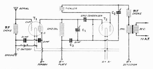
Fig. 1: How a stage of untuned radio-frequency amplification is added to the familiar straight regenerative tuner. The connections are shown only up to the detector, as the audio system remains unchanged.
