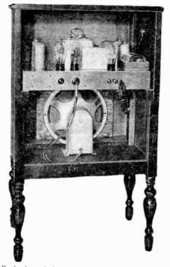
Back view of the Pilot 10-tube Console, showing the arrangement of the chassis and the mine-inch dynamic speaker.
