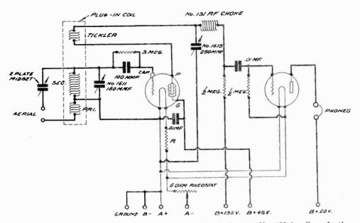
Hook-up of a two-tube short-wave regenerative receiver using the No. 180-4 coils. Another audio stage may be added if loud speaker results are desired.
