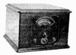
The short-wave converter of the "All-Wave" is available as a separate unit, which may be used with any broadcast receiver, regardless of type. It makes short-wave reception comfortable and easy.
