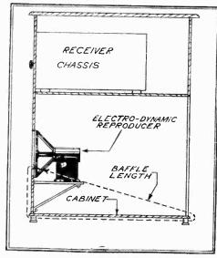
Fig. 3: How the front and sides of a cabinet act as balle for the loud speaker.
