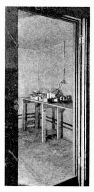
Looking through the door of the "Torture Chamber" into the iron-lined inside. Two receiver chassis are on the table undergoing a heat and humidity test.
