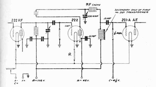
This diagram shows how a screen-grid detector is used in the K-110 model Super-Wasp. The rest of the R.F. and A.F. connections remain the same as before.
