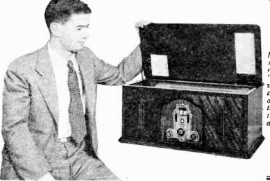
His Majesty's personal short-wave receiver, a Pilot "All-Wave". The white areas on the cover are pieces of asbestos that protect the wood from the heat of the 280 and 245 tubes.
