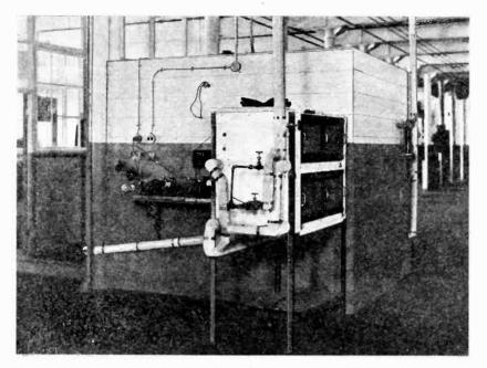
Back view of the "Torture Chamber," with the separate condenser over in the foreground.
