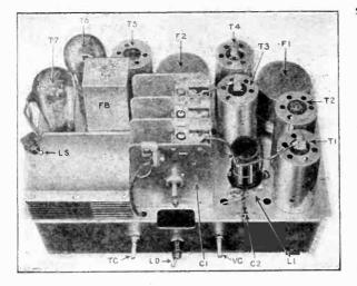
A close-up of the seven-tube super-heterodyne chassis, with all the parts marked to correspond with the designation on the schematic diagram on the next hage.
