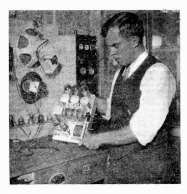
Mr. A. M. Morgan, of the Pilot engineering staff, showing the chassis construction of the TRF Midget. The RF transformers for the 200-550 meter range are in the shield cans next to the threegang tuning condenser.
