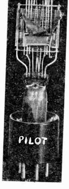
Left, Fig. 1: a broken-down view of the 247 power pentode tube, showing the multiplicity of grids between the plate and the filament.
