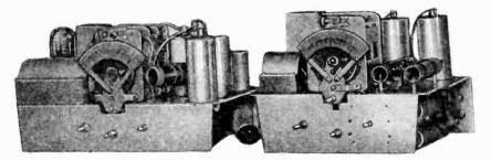
The chassis of the "All-Wave" out of the cabinet. Left, the 7-tube broadcast unit; right, the four-tube short-wave converter. Four of the coils of the latter unit are visible at the extreme right.
