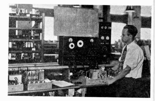
Above, Fig. 4: The ingenious continuity testing board, which indicates the condition of every circuit in a receiver. After a set comes off the assembly line it is passed on to this board before it goes to the shielded test booths. Minor errors in wiring or adjustment are quickly detected, and the necessary repairs made without delay.
