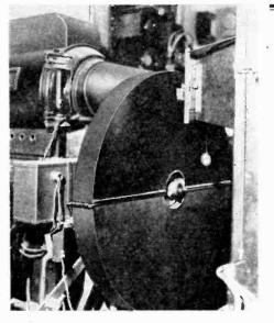
Above: A close-up of the enclosed scanning disc used in the W2XBS television transmitter. Behind it is the arc light, and in front the opening in the frame that holds the photoelectric cells.
