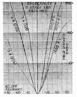
tune in any broadcast station without a trace of interference from stations on adjacent channels. Furthermore, the selectivity is uniform at all broadcast frequencies.
