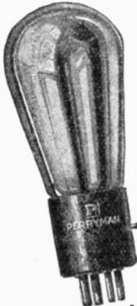
Type P.A. 210 Super-power Amplifier New Standard base with long pins
