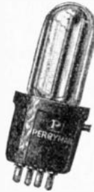
Type R.H. 199 Amplifier-Detector Adapter Base with short pins
