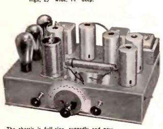
The chassis is full-size, ruggedly and powerfully built. It is 17 inches wide, 11 inches deep and 10 inches high. It uses one UY 227 oscillator, four UY 235, super-control screen grids, two UX 247 power pentodes and one UX 280 full wave rectifyer. A full 12 inch Jensen Dynamic speaker gives superb quality on both low and high notes.
