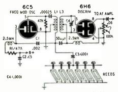
Fig. 3-Author's circuit needs no shielding.
