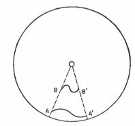
Fig. 3—Pinch Effect cause near disc center.
