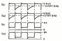
Fig. t-b-Plate and grid voltage wave forms.
