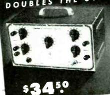
Gives two separately controllable traces individual inputs on any scope. See both the input and output traces, locate distortion, phase shift, etc., immediately. Individual gain controls and positioning control. Coarse and fine sweeping rate controls. Complete Heathkit matches others, with 5 tubes, All metal parts are punched, formed and cadmium plated. Complete with tubes, all parts, detailed blueprints and instruc-
