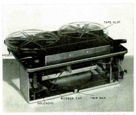
Fig. 3—Another view of the tape-handling mechanism, with protecting hoods in place.
