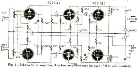
No construction details are given, as any exactly similar pair of amplifiers may be used.
