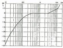
Fig. 2—British discs are recorded this way.
