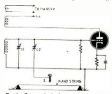
Fig. 2—One method of using FM for piano.
