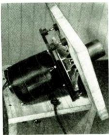
Fig. 5-Suction source is rotating impeller.
