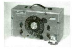
MODEL 906 FM-AM SIGNAL GENERATOR. Similarly the choice of the big engineering laboratories plus thousands of service technicians, 906 stands out as maximum value. 90 kc. thru 210 mc. in 8 ranges, ±1% accuracy; less than ½ microvolt, including strays to over 1 volt v.t.v.m.-metered output; multiple shielding; adjustable 0 to 1,00% amplitude modulation; adjustable 0 to 1,000 kc. FM sweep. Net price only \$116.50.
