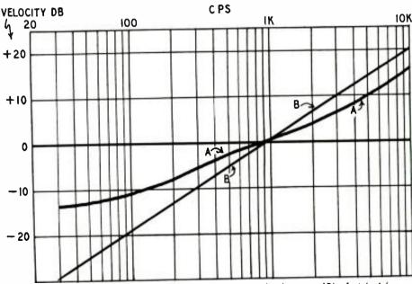
Fig. 6-Microgroove recording curve (A) vs. constant amplitude curve (B) of xtal pickup.
