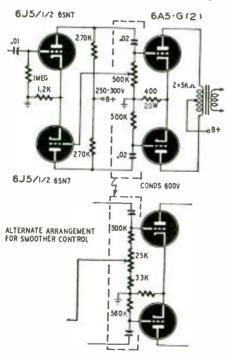
Fig. 1—Old Standard phase-inverter circuit.
