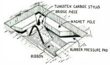
Fig. 1-Details of new Brierly ribbon pickup. sired response near the start of the grooves, the upper a.f. limit halfway to the center would be a whole octave lower.
