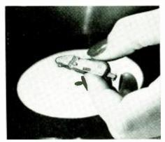
The ceramic crystal pickup made by Sonotone.
