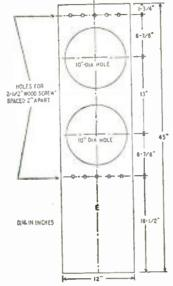
Fig. 3—Detail of one of the speaker boards.
