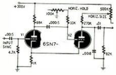
Fig. 4 Typical cathode-coupled multivibrator.
