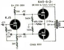
Fig. 3-Split-load inverter uses single tube.
