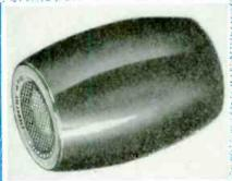
The Stephens C-I is a new condenser microphone that phase-modulates a crystal oscillator. Response extends from one-half cycle in 24 hours upward to 15 kc.
