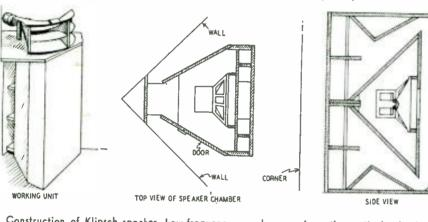
Construction of Klipsch speaker. Low-frequency sound comes from the vertical side slots.
