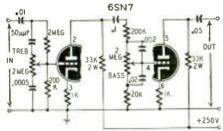
The equalizer controls both treble and bass. ficient reserve voltage gain.
