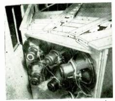
Fig. 2—How the six speakers are mounted.
