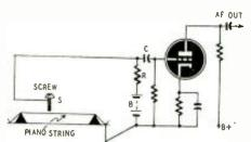
Fig. I—Older pianos used polarizing voltage.
