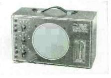
MODEL 905-A "SPARX". Combining signal-tracer and universal test speaker, 905-A is amazingly sensitive yet free af usual tracer hum. Vacuum-tube prod with r.f.-a.f. switching; high-gain high-fidelity amplifier; 6" PM speaker; 18-watt output transformer gives wide choice af impedances. Two essential instruments in one, 905-A is the finest 37 years of prize-winning radio engineering experience can design — value far exceeding \$44.50 net.
