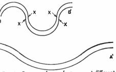
Fig. 4—Grooves of same frequency at different disc diameters.
