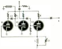
Fig. 1-The LC circuit serves to time pulses.
