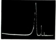
Fig. I-A 1.5-kilocycle wave and harmonics.
