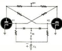
Fig. 5-a-The direct-coupled multivibrator.
