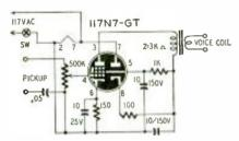
is used. No tone control was found necessary, but if one is desired, a capacitor and 1-megohm variable resistor may be placed in series between the amplifier grid and common negative.
