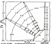
Fig. 1-Floor plan of triple speaker system.
