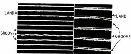
Fig. 1, left; Fig. 2, right—Photomicrographs of ordinary and Microgroove record section. Owing to variations in records, the ratio is nearer 2:1 than the more usual 3:1.
