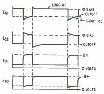
Fig. 2-Wave forms in an unbalanced circuit.
