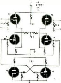
Fig. 7-Double-tracker for an oscilloscope.
