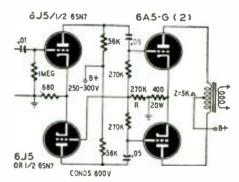
Fig. 2-R should be large for best balancing.
