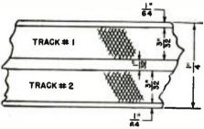
Fig. 1—How the two tracks are positioned.
