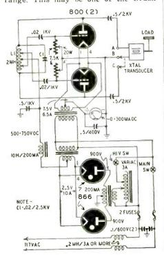
Development Co. Models AX-171, AX-178, AX-180 or equivalent. Be sure that the model you select can handle the power you develop in the generator. There are three output terminals. Connect the transducer across any two of experimental circuit constants?-J.E.G., them. The ones you use depend on the type and operating limits of the trans-
