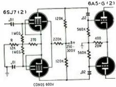
Fig. 4—Cathode-coupled inverter works well.
