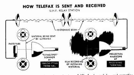
This highly simplified diagram shows the main steps of Ultrafax transmission and reception.
