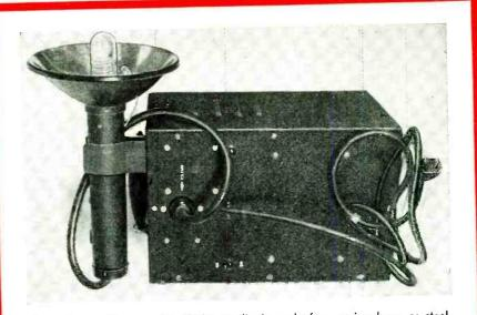
Front view of the case. The flash-gun clip is made from spring brass or steel.
