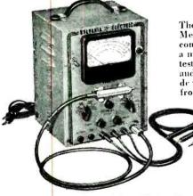
The Sylvania Poly (MULTI-PURPOSE) Meter Type 134Z provides, in a single compact instrument, the means of making a multitude of electrical measurements and tests. Electrical values measured include audio, ac and rf voltages (up to 300 mc); dc voltages from 0.1 to 1,000; direct currents from .05 milliampere to 10 amperes; resistances from ½ ohm to 1,000 megohms. Instrument is compactly built, at-
