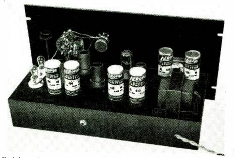
The balance adjuster RI can be seen at the upper left. Knob is attached to the long shaft.
