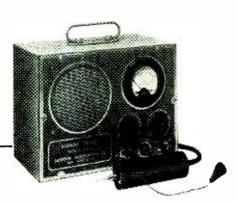
S IGNAL tracing has for some years been the accepted method of quick, mass-output trouble shooting in radio receivers. The radio technician prefers to use it to localize defects quickly. Then he may apply other equipment to discover the defective part or incorrect condition.
