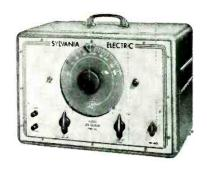
This Audio Oscillator Type 145 is one of the most versatile and convenient test instruments made. Its powerful signal of known frequency provides an accurate tone source for checking radio receivers. It is ideal for response and distortion testing of audio amplifiers, public address systems, juke hoxes, wired music installations and individual speaker cones. An exceptionally valuable test instrument. Price: \$129.50.
