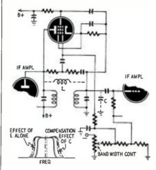
When the bandwidth control (see figure) is set near the grounded end, the gm of the reactance tube is high. This results in a higher  $I_D$  for a given  $E_g$  and is equivalent to a lower effective L and more loading across this effective inductance. The lower inductance increases the coupling between stages, but the double-hump response does not appear because of the added loading. The bandwidth variation is also accompanied
