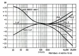
Fig. 2—Responses obtained with the main equalizer controls.
