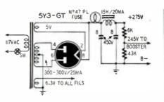
Fig. 3—The booster diagrammed above is powered by the simple supply shown here.
