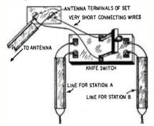
Fig. 4-A switch selects desired tuning line.
