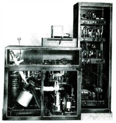
Photos courtesy Process & Instruments Rear of commercial mass spectrometer. Note curved tube and vacuum pump.
