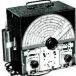
Signal Generator Specifications: Signal Generator Specifications: \*Frequency Range: 150 Kilo-cycles to 50 Meracycles. \*The R.F. Signal Frequency is kept completely constant at all out-put levels. \*Modulation is ac-complished by Grid-blocking ac-tion which is equally effective for alignment of amplitude and frequency modulation as well as for television receivers. \*R. F. ob-tainable separately or modu-lated by the Audio Frequency. Shamal Tracer Specifications:
