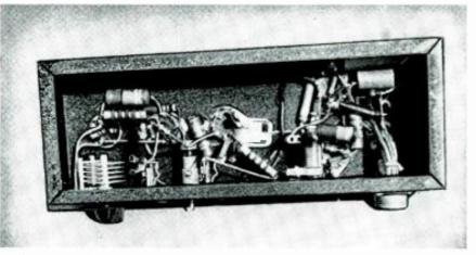
This is the underside of the transmitter chassis. Final tank tuning capacitor is at left.
