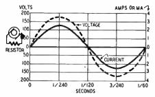
Fig. I—E and I in a resistance are in phase.
