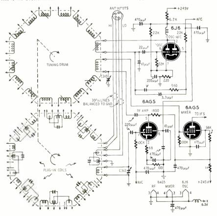
Fig. I—Original circuit of the Philco television tuner. Coils may be had for any channels.
