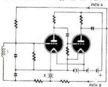
feedback voltage to the cathode. Therefore, at the crystal frequency, there is no negative feedback and the circuit oscillates only at this frequency.
