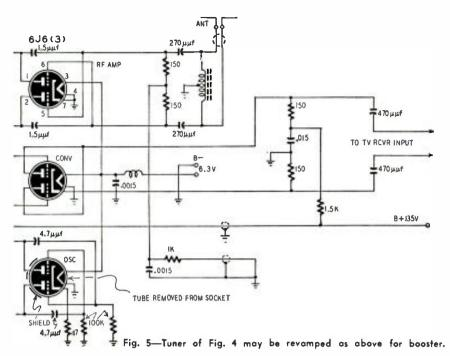
neater job. Take care not to open circuits unintentionally, because some ground or B-plus returns may be terminated at the oscillator-tube socket.
