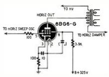
Fig. 3-Remove 0.1-µf screen-grid capacitor.
