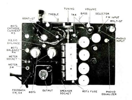
The 11 x 17 x 3-inch chassis holds the push-pull 807 amplifier in addition to t.r.f. tuner.
