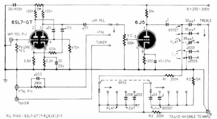
This amplifier control unit, with its volume and equalizer controls, is on a  $10 \ge 4 \ge 2\frac{3}{4}$ -inch chassis that can be mounted in the cabinet of a large record player. Suggested by a circuit in *Radio and Hobbics* (Australia), it consists of a 6SL7-GT compensated preamplifier for variable-reluctance magnetic pickups and a straight 6J5 amplifier designed with a gain of approximately 14 to compensate for the losses in its plate equalizer circuits.
