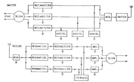
system the Selsyn output voltages are rectified. filtered, and used to control separate audio oscillators. As an example, these may generate 60, 120, and 240 cycles, respectively. The amplitude of each will depend upon the Selsyn output which controls it. Each of these audio voltages is fed
