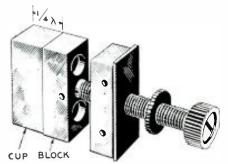
Fig. 6-The cup-type plunger reduces losses.
