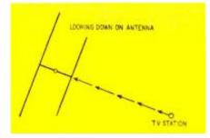
Fig. 1—Antenna is broadside to the station. RADIO-ELECTRONICS for
