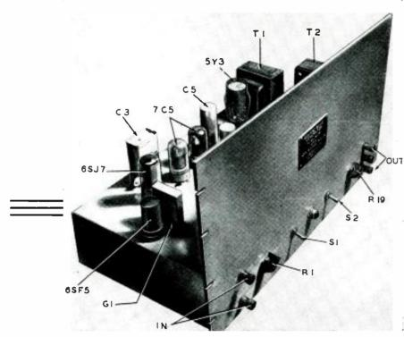
Square waves at frequencies up to 50 kc may be produced with this instrument plus an a.f. generator
