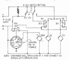
Simplified schematic of the PE-103 dynamotor.
