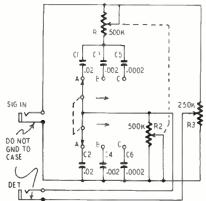
Fig. 3—Schematic of a practical Wien bridge. shown. If wired backward, as in Fig. 4-b, the frequency calibrations will be
