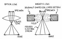
Fig. I—Magnetic field focuses electron beam.
