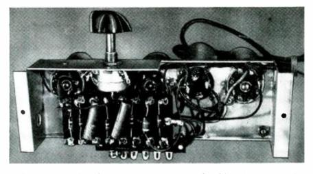
The few components, if wired point to point as in commercial models, make unit inexpensive.
