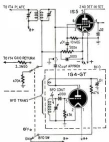
increase the tuning range to 36 mc if you desire 10-meter reception. A twogang, 35-µµf capacitor can be connected across the main tuning capacitor to provide bandspread tuning.
