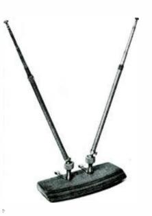
The antennas used are commonly available on the surplus market. However, if these are not obtainable, collapsible automobile antennas can be used. The ball-and-socket fittings, purchased from a hardware supply house, are similar to those used on some types of casement windows. We used hardwood for the base. Any insulating material will work just as well. The underside of the base should be covered with a layer of felt or fitted with small rubber feet.
