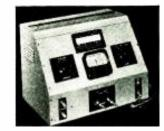
ond groding capacitors. It may be used by nan-technical personnel to obtain results within 0.2%. The range of the reading is 10 µuf to 1,000 µt. The meter is a 4-inch direct-current D'Arsonvol is a type.
