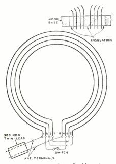
Fig. I-Connections of the fixed-loop transpole television antenna. Construction inset.
