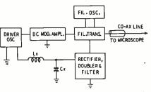
Fig. 5-Block diagram of 60-kv power supply.
