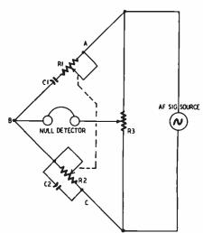
Fig. I-Basic Wien frequency bridge circuit.
