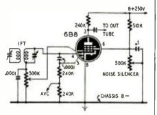
The screen voltage is supplied by a voltage divider consisting of a 240,000ohm resistor and a 500,000-ohm potentiometer. This control can be adjusted to a point at which noise cannot exceed the signal level.
