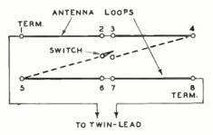
Fig. 2—Simpler diagram explains unit above.
