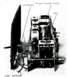
Chassis photo shows tuner, safety interlock.
