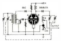
coil of triode A. Tank D tunes the doubler stage, triode B. The two tuning capacitors may be gauged as usual for single-dial tuning. A and B may be separate triodes or a double triode such as the 7Fs.
