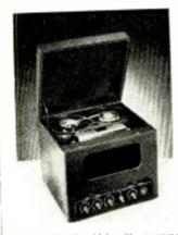
Model CL-10, which will accommodate messages from 4 seconds to 10 minutes, aperates on the same principle, but utilizes a storage system with lower inherent friction, accomplished through the use of ball-bearing rollers. Either model can be adapted for automotic recycling, a system which sets the Twin-Trax recorder in RECORD position when the press-to-talk switch of the microphone is operated. Release of the switch resets the instrument into PLAY position.
