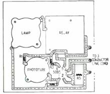
Fig. 2—The base layout and "wiring diagram."
