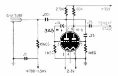
Fig. 3—Tube is quenched by a negative pulse.
