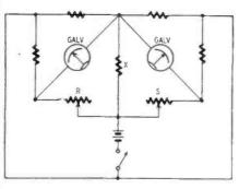
recently developed double bridge saves time by allowing both limits to be checked at the same time by using two galvanometers and two bridges, connected as shown. The unknown resistor X is common to both bridges. Variable elements R and S are adjusted to the required limits, for example + 5% and 5%, respectively. Each meter is calibrated in terms of REJECT and ACCEPT. If both indicate ACCEPT, the resistor is within its limits
