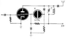
There are two main adjustments to be made on the final stage of a transmitter. The first is to align the preceding stages so that maximum power is delivered to the final grid. The second is to resonate the final plate. Both can be done with the aid of a neon lamp N connected as shown.
