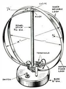
Fig. I—Construction details of variotenna.
