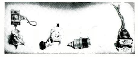
Typical tuned circuits: wavetrap, high-frequency receiver tank, slug tuner, transformer.
