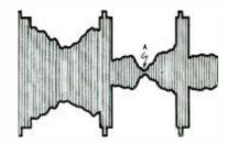
Fig. 5-Zero video modulation blanks sound.
