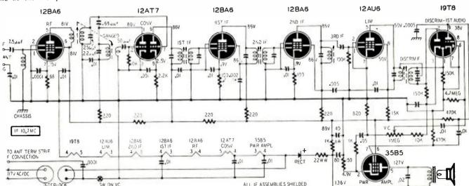
Complete circuit schematic of the Zenith 7FO3 FM receiver chassis. The single limiter does a good job, even in a noisy New York location.
