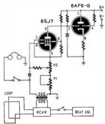
The detector is direct-coupled to one section of the indicator tube. The other is not used; therefore its control element is connected to B-plus through a resistor which drops the voltage just enough to close its corresponding shadow.
