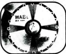
Fig. 3—Too much contrast causes effect at left. Compare with normal contrast at right. film recordings of the actual studio programs are not made instead of photographing the image on the cathoderay tube monitor. Obviously, many of the critical factors encountered in reeording from the monitor would thus be eliminated.
