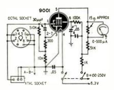
There being no circuits to tune, the device checks crystals regardless of frequency. A three-prong crystal socket and an octal tube socket are wired to take most of the available crystal holders. Operating voltages may be taken from any convenient source.
