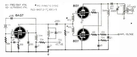
Fig. 2—A larger ultrasonic generator using a quartz crystal ta praduce the vibrations,
