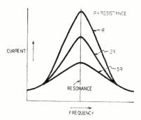
Fig. 3—Resistance effect on series circuit.
