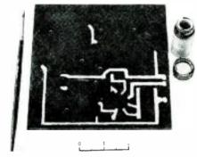
Fig. 3—The board with conducting lines drawn.
