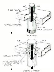
Fig. 4—Four waveguide-to-co-axial sections.
