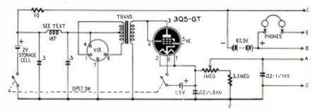
Fig. I—This is the schematic diagram of the power-supply components inside the main case.
