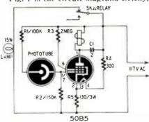
Fig. I—Schematic of the phototube circuit.
