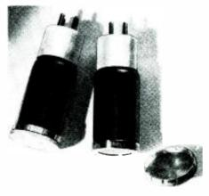
Tracerlab tubes with removable beta shields.
