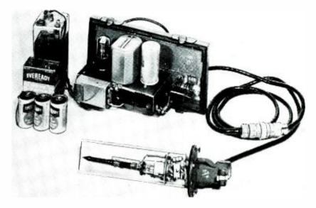
Photograph of complete instrument disassembled shows inside of probe and top of chassis.
