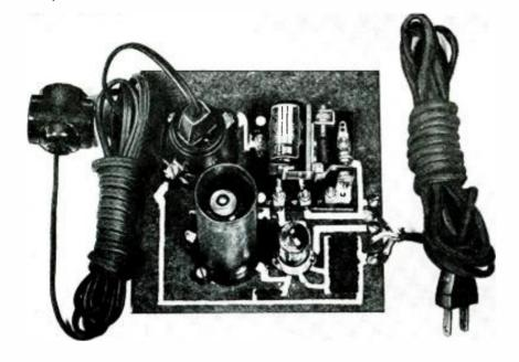
New kit of paints allows experimenters and development engineers to make their own printed circuits, obviating need for special equipment
