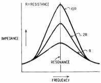
Fig. 6-Resistance lowers Q of parallel tank.
