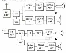
Fig. 1-Intercarrier and standard contrasted.
