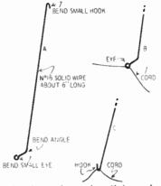
tion. B shows how the dial cord can be threaded through the eye and carried wherever you want it without the danger of its dropping into some hardto-get-at place. Drawing C shows how the hook can be used to retrieve the cord from a tight spot.
