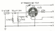
Fig. 2—G-M tube and amplifier are in probe.
