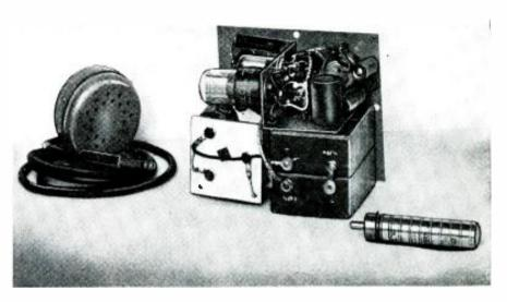
The Farty-Niner disassembled, showing power supply-amplifier, shoulder speaker, G-M tube.
