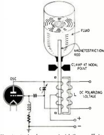
Fig. I—A simple magnetostriction oscillator,
