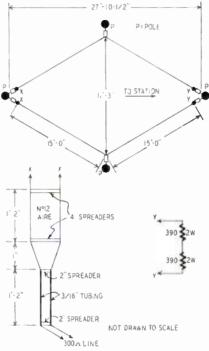
should be mounted in a small water-proof container and connected across the end of the antenna nearest the TV station.
