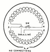
Fig. 3-Wiring for the Inductive Tronspole.
