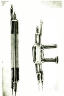
Courtesa N. Wood Counter Laboratory A pair of laboratory-type Geiger-Muller tubes.
