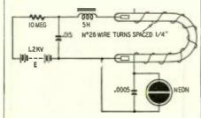
The diagram shows a flasher operated from a high-voltage dry battery. The .015-µf capacitor is charged through the high resistance; and when a critical potential is reached, the U-shaped neon lamp flashes. Then static accumulates on its glass envelope.
