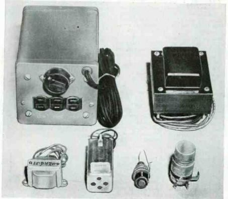
Some of the many types of transformers used in radios. Rear we have an isolation and a power transformer. Front, an output, an i.f., iron-core r.f. and an antenna transformer.
