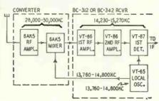
Fig. 1—Converter precedes BC-312 front end.
