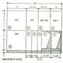
Fig. I—How to loy out the sheet of plywood.
