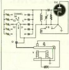
ess series capacitance is used in series with C1 at the upper channels to reduce the relative frequency deviation
