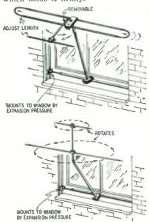
Fig. 7—Two easily-mounted window antennas.
