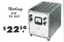
Now a bench 6 Volt power supply kit for all auto radio testing. Supplies 5-7½ Volts at 10 Amperes continuous or 15 Amperes intermittent. A well filtered rugged power supply uses heavy duty selenium rectifier, choke input filter with 4,000 MFD of electrolytic filter. with 4,000 MFD of electrolytic inter.
