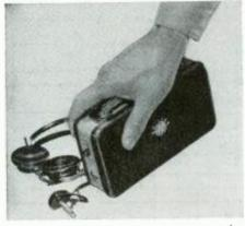
Nuclear "Sniffer" uses vibrator power supply.
