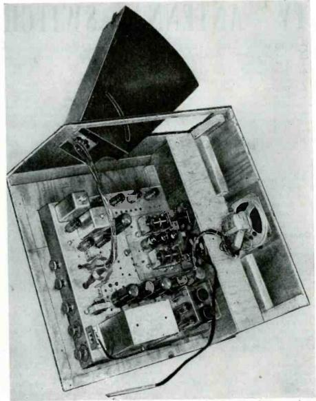
Back, bottom, and left side of ccsa are removable in a single unit for adjusting receiver.
