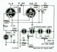
Fig. 3—Relaxation oscillator feeds the 1L4.
