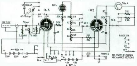
Fig. 2—The neon lamp in the El-Tranics SM-3 limits the amplitude of the pulses reaching V2.
