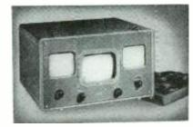
antenna included with receiver. Allchannel tuner has fine-tuning control, 18 tubes, 4 rectifiers. A.c. operation only. Weight, 28 pounds. (John Meck Industries, Inc., Plymouth, Ind.)
