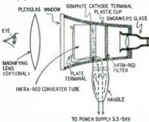
Fig. 2-The construction of the snooperscope.
