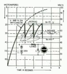
Fig. 2—Curves show action of the oscillator.
