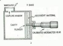
Fig. 3-b—A variable-frequency cavity meter.
