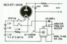
Fig. I-Miniature high-voltage power supply.
