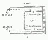
Fig. 3-a—A fixed-frequency cavity wavemeter.
