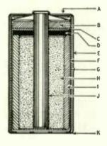
Alpha Leclanché cell. A—double-sealed metal top; B—plastic seal; C—wosher; D—expansion chamber; E—metal shell; F—seamless zinc can; G—moisture-proof bitumen boord; H—depolarizing core; I—paste electrolyte; J—carbon electrode; K—the metal bottom reinforcement.
