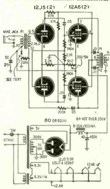
Fig. I—The amplifier for carbon microphone. RADIO-ELECTRONICS for
