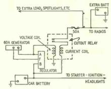
regular battery. A standard 60-ampere generator is adequate for charging both.
