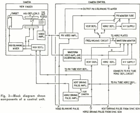
HE immediate output signal of each camera is usually below the quality standards of the station, or may differ from the exact needs of the particular program. To compensate for these differences a chain of electronic devices is employed. The first of these, the electronic viewfinder, is directly attached to the camera by plug and socket connections.
