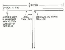
Fig. 1-Correcting the "half-wave" dipole.
