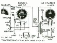
Fig. 2—Replacing resistors increases output.
