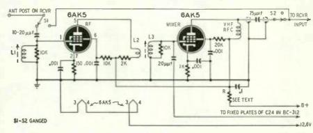
Fig. 2—The 10-meter converter is a broad band r.f. amplifier. Receiver acts as variable i.f.
