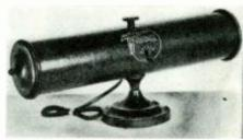
Fig. 5-b-Cylindrical antenna with tuning.
