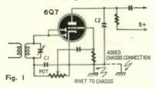
The next step was to try all the soldered joints and contacts with a screwdriver. On touching the cathode contact of the 6Q7, the hum stopped suddenly. Yet this electrode was connected to chassis with but a scant 1/2 inch of bare wire. We checked the soldered joint to the rivet which held the tube socket to the chassis and which was used as the chassis ground (see Fig. 2).
