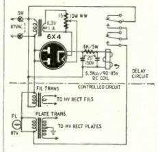
The rectifier must reach operating temperature before it will pass enough current to throw the relay; therefore the delay interval is equal to, or slightly less than, the warm-up time. Since warm-up time is determined by the applied heater voltage, the delay interval can be increased by decreasing the heater voltage. Heater voltage is controlled by the setting of the tap on the 5-ohm, 10-watt resistor across the secondary winding of the filament transformer
