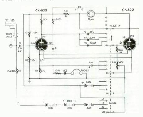
Fig. I-Pulses furnished the meter deflect it in proportion to the frequency of the pulses.
