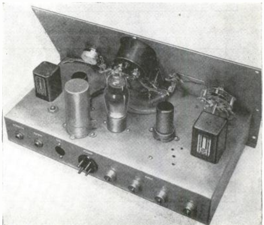
Photo shows chassis and panel pulled out of cabinet. Male power connector is used for safety.
