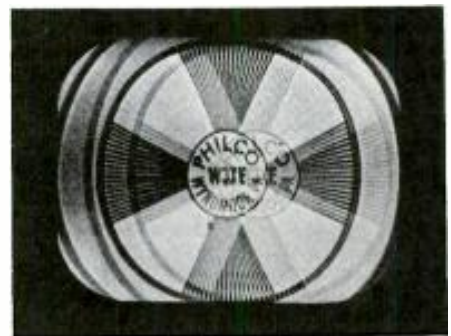
These photos of television screen show typical results of an incorrectly oriented antenna.
