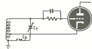
Fig. 5—For correct tracking, a padder capacitor is placed in series with the tuning capacitor as in this circuit.
