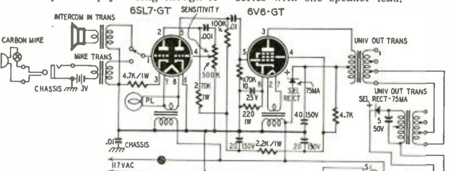
Fig. 4—Schematic of the sound switch. The thermostat-controlled time delay is varied by adjusting the variable contacts of the thermostat or by R1.
