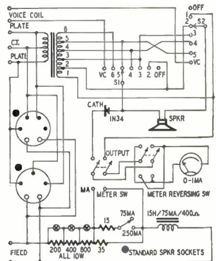
Schematic of the loudspeaker test set.
