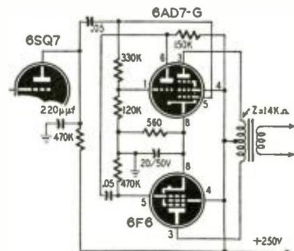
Fig. 2—Circuit of the push-pull stage. current of the push-pull stage in Fig. 2 is approximately 53 ma. If the power transformer in the set is not already operating at top capacity, the added drain should not cause overheating.
