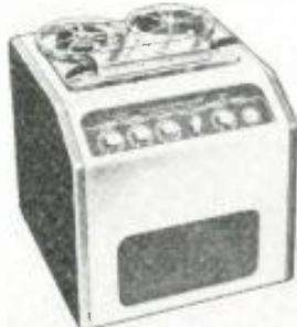
or low impedance microphones. Input mixing circuits are optional. A 6ES volume level indicator is built in and jacks are provided for connecting an external VU meter.
