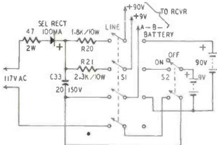
so the voltage applied to the filament string does not exceed 9 volts under load. We suggest using a 2,500-ohm, 10-watt resistor with slider in this position. Codes on the components correspond to those in the original circuit.
