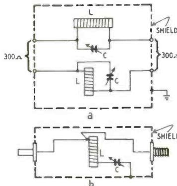
Fig. 3—Shunt- and series-tuned traps.
