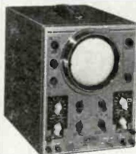
The sweep oscillator provides a saw-tooth wave from 20 cycles to 50 kc in 5 steps. A 60-cycle sine wave sweep is also available. Direct connection, through capacitors, can be made to the C-R tube deflection plates. A demodulation probe to use for signal tracing in television or radio receivers is also available.
