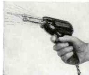
considerably smaller and lighter than the previous 135-watt models. Other features are dual heat (100/135 watts), 5-second heating time, trigger-switch control which adjusts heat to the work, and a chisel-shaped tip for faster heat transfer and speedier soldering. The tip is replaceable.
