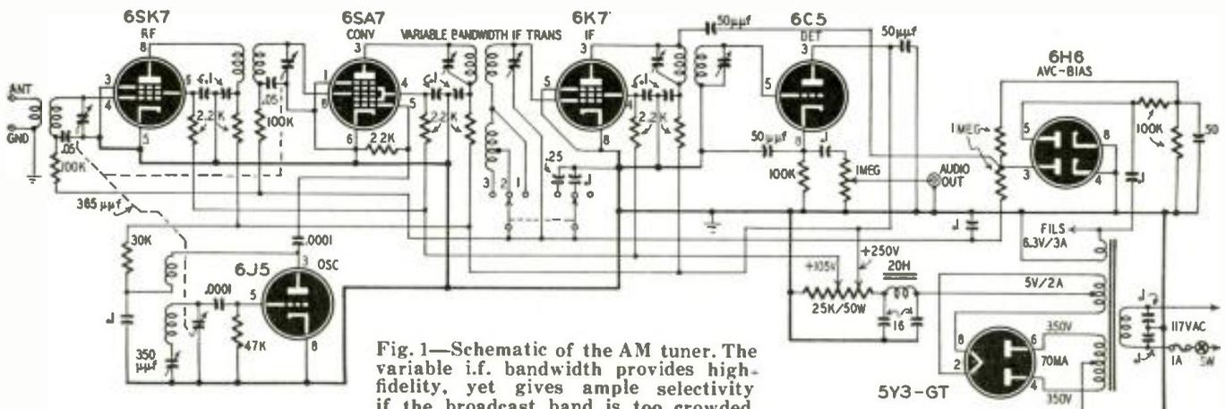
Fig. 1—Schematic of the AM tuner. The variable i.f. bandwidth provides high-fidelity, yet gives ample selectivity if the broadcast band is too crowded.
