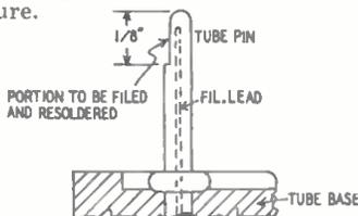
Failure of the 1B3-GT rectifiers can often be traced to poorly soldered connections the filament leads and the tube base pins. These tubes can be repaired and returned to service by filing pins 2 and 7 as shown in the drawing and resoldering them with noncorrosive solder which is allowed to flow freely to insure good connection.—Philco Television Service Bulletin
