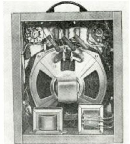
At left is a front panel photo of the portable loudspeaker test unit. Above is a rear view of the unit.
