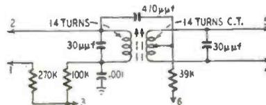
cuit. Instead of using a capacitive center tap on the secondary of the transformer, he has center tapped the winding and has changed the coupling capacitor from 22 to 470 µf.
