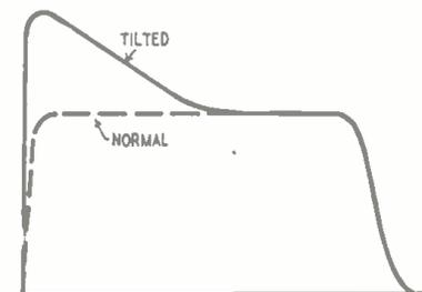
Fig. 5—Video response curves showing effects of raising low-frequency gain.
