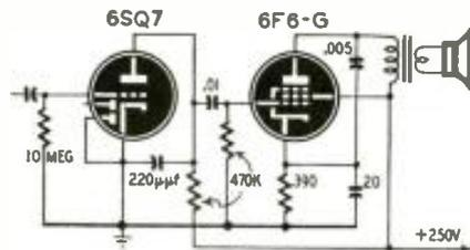
Fig. 1—The audio circuit of the T-64. the corresponding circuit of an RCA model QU2C receiver. The 6AD7 is a triode and power amplifier pentode in a single envelope. The pentode section is equivalent to a 6F6. The triode section is designed as a phase inverter to drive the push-pull stage.
