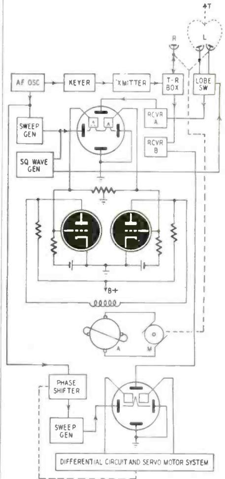
Diagram of the radar system. The size or position of the pips on the scope screens controls the two servo systems.
