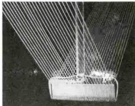
bars. The photo shows one corner of an all-plastic loop antenna using 1/2-inch diameter Lucite rods for the cross-members. If desired, the teeth can be shortened by clamping the combs in a vise and sawing through the row of teeth carefully.—Arthur Trauffer
