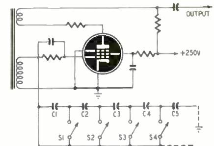
Fig. 2—In this circuit a series combination of capacitors is selected to get the desired pitch. When all of the switches are open the pitch is highest.
