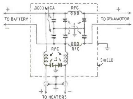
duce the hash as much as possible by cleaning the brushes and commutator. Construct a small r.f. filter as shown in the diagram and install it close to the dynamotor. The r.f. chokes may be 20 turns of No. 12 insulated wire close-wound on a 3/4-inch form. The filter should be installed in a small metal box or shield can. Try connecting it to a good ground. Use heavy leads in the 6-volt circuit to minimize voltage drop.
