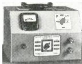
amps. The output is variable from 0 to 15 volts d.c. A 10,000-uf capacitor provides the filtering. The rectifier has a full-wave bridge circuit using 4 heavy duty manganese copper-oxide rectifiers.
