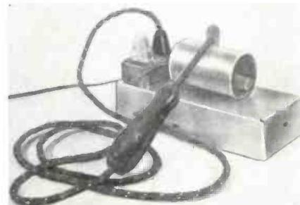
Photo of the soldering iron regulator.
