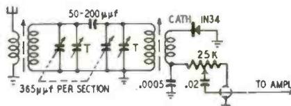
tenna coils connected back-to-back through a coupling capacitor which may be between 50 to 200 µf. The secondary windings are tuned by a two-gang, 365-µf tuning capacitor.
