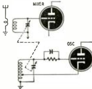
Fig. 4—In the superhet, the oscillator and mixer tuning capacitors are on one shaft as indicated by the dashed line.
