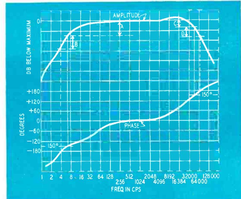
Fig. 2—Typical amplitude and phase characteristics of an audio amplifier.
