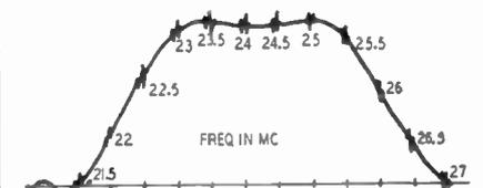
Fig. 5—With both crystals in operation the over-all response curve shows accurate marker pips every half-megacycle.
