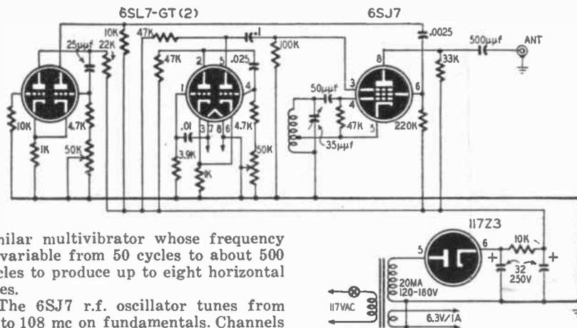
similar multivibrator whose frequency is variable from 50 cycles to about 500 cycles to produce up to eight horizontal lines.
