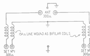
Fig. 2—An efficient two-set coupler.
