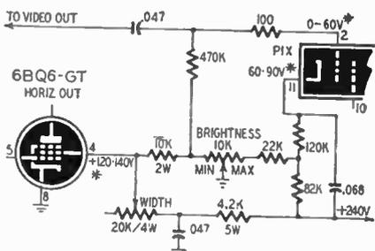
Fig. 6—Automatic width-control circuit in some recent Philco television models.
