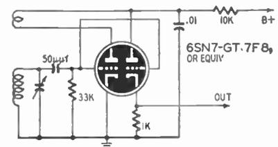
Fig. 1—Oscillator-buffer arrangement.
