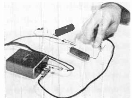
How it is set up to check a capacitor.
