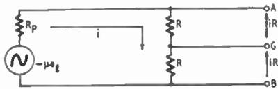
Fig. 1—The best type of phase splitter, shown above, is simply two resistors with their junction grounded. The voltages have to be equal and opposite as long as the two resistors maintain their equal resistance. This circuit also has some practical applications.
