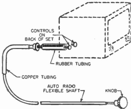
trol shaft, a length of copper tubing, and a short piece of windshield-wiper hose. The copper tubing controls the degree of bend to prevent whipping and binding. The rubber hose slips over the shaft of the control to be adjusted.—*Motorola Service and Installation Bulletin*
