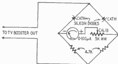
are connected in series across the output of the bridge. The reading of the meter is proportional to the strength of the signal fed into the booster. The 5,000-ohm calibration control permits the meter to be set to a predetermined reference point. Silicon diodes are more efficient at TV frequencies than most germanium types.
