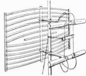
channels, good front-to-back ratio on all channels. The antenna can be tipped to shift the vertical pattern without tilting mast and can be used with antenna rotator. It is 6 feet, 2 inches high (less mast), 8 feet wide, and 4 feet deep.
