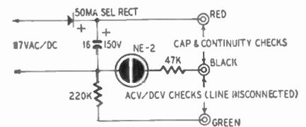
Fig. 1—The checker uses few parts.
