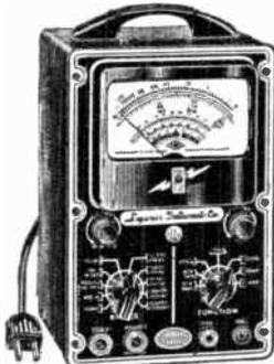
Comes housed in rugged, crackle-finished steel cabinet complete with test leads and operating instructions. Size 6 1/4" x 9 1/2" x 4 1/4".
