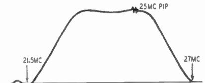
Fig. 3—Typical i.f. response curve with 25-mc marker pip from crystal calibrator.
