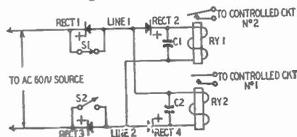
rectifier 2 conducts because its anode is positive. These two rectifiers pass current through relay 1 and cause its contacts to operate. Relay 2 operates when S2 is closed. Both relays operate when S1 and S2 are closed. C1 and C2 may be of any value large enough to keep the relays from chattering.
