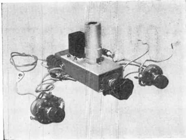
Photo C—A top view of the finished calibrator. The output controls and on-off switches are at the ends of flexible leads.
