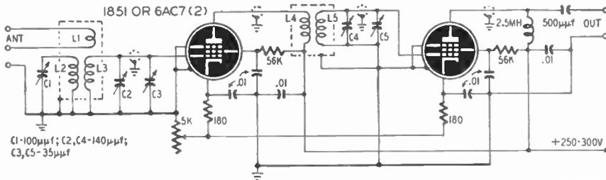
ground end of L3. Spacing between L1 and L3 is 5/32 inch for 200-80 meters, 1/8 inch for 80-40 meters, 1/4 inch for 40-20 meters, and 1.8 inches for 20-10
