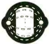
*This illustration clearly shows that the concentrated field of energy between the two conductors, which are 7 strands of #28 copper weld wire, is contained by the tubular construction. This important field of energy is unaffected by any exterior conditions.*
