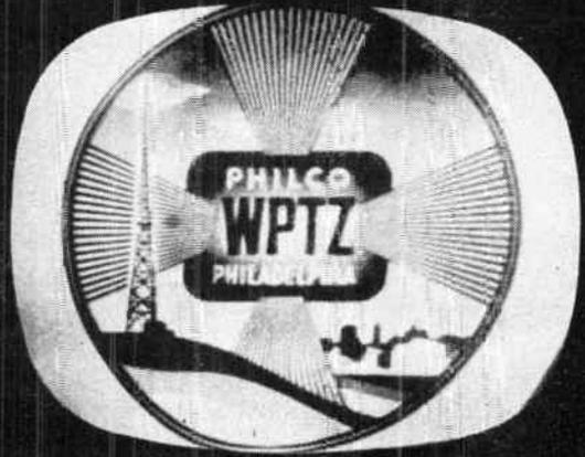
Appearance of screen when cosine yoke is used without the corrector magnets.
