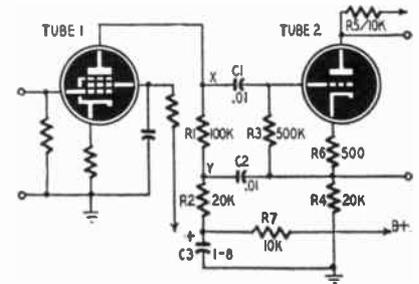
Fig. 7—This more refined circuit overcomes the reduced gain by taking advantage of the cathode-follower circuit's high input impedance. By using a pentode in the first stage, the combined gain of the two stages is excellent.
