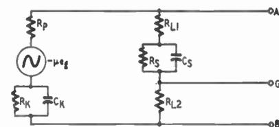
Fig. 4—How the circuit of Fig. 3 appears to low audio-frequency signals.
