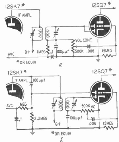
Fig. 3—(a) Standard a.v.c. circuit. (b) Modification for less distortion.
