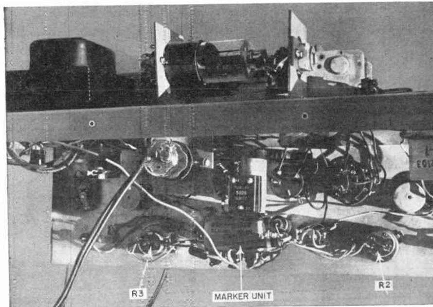
Photo D (below)—The marker unit installed below the chassis on the panel of a Heathkit model TS-2 sweep generator.
