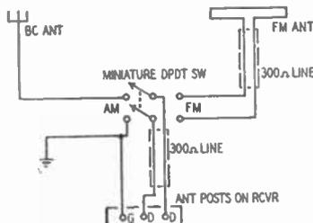
of the D (dipole) terminals. The short is removed and the 300-ohm lead-in connected when the switch is thrown to FM. I used a switch mounted on an insulated block measuring only 1 x 1 1/4 inches. The spacing between its blades is only 1/2 inch. This preserves the symmetry of the 300-ohm ribbon and minimizes reflections and mismatch. The switch is mounted on a polystyrene angle bracket at the rear of the receiver.—Arthur Trauffer
