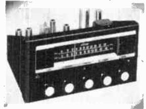
The C800 has a total complement of 15 tubes and can be mounted in the same panel formerly cut for an RC10 or C10 tuner.
