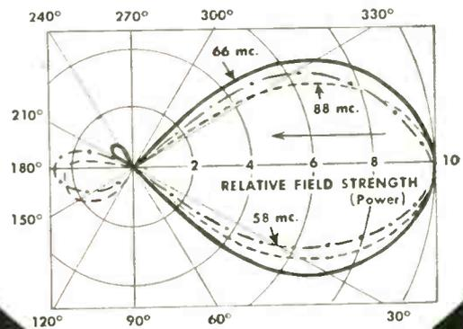
The test patterns on both high and low bands reveal the Amphenol Inline Antenna's superior uni-directional reception lobe. This single forward lobe intercepts the TV signal at its maximum available strength. It also rejects unwanted reflected signals or side interference that cause “ghosts” and unsteady pictures.
