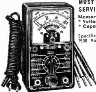
Handsome round cornered molded bakelite case 3 1/4" x 5 7/8" x 2 1/4" complete with all test leads and instructions
