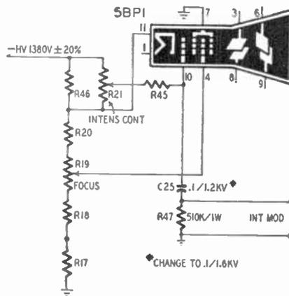
resistance drops when voltage is applied. This places an excessive drain on the high-voltage supply and causes a high negative voltage to appear across the INT MOD terminals.
