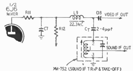
Fig. 1—How a sound take-off and trap can be installed in the cascode tuner.
