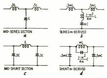
Fig. 3—Basic low-pass filter sections, with corresponding m-derived types.
