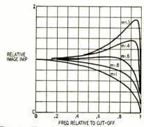
Fig. 5—How image impedance of lowpass filters varies with different m values.
