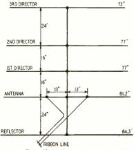
Fig. 2-Details of a channel-4 Yagi. RADIO-ELECTRONICS
