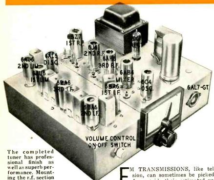
M TRANSMISSIONS, like television, can sometimes be picked up far outside their estimated useful service areas. Today, thanks to recent developments widely used in television receivers, it is possible to build an FM receiver which has the high sensitivity and extremely low noise level necessary to give consistent, satisfacThree low-noise r.f. stages and bandpasscoupled i.f.'s solve a receiving problem
