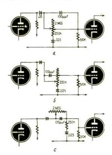
The control circuit consists of a 2.5megohm potentiometer tapped at 250,-000 ohms and two capacitors. The control network is used between two highmu triodes.
