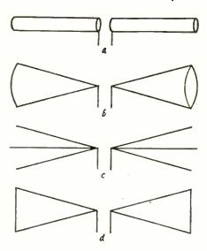
Fig. 7—(a) Increasing diameter of elements increases bandwidth. (b) Biconical dipole covers wide frequency range. (c) Fan-dipole form of conical antenna. (d) "Bow-tie" solid-sheet dipole for u.h.f.
