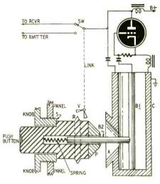
The figure shows a coaxial-line cavity. the grounded outer conductor. B1 is the inner line which has an extended portion B2 passing through a flared aperture in C. A metallic, tapered plug P fits snugly into this aperture A, when the push-button is depressed. When desired, a catch (not shown) is set to hold the plug in this position. When P is inserted into A, the oscillator frequency is the natural frequency of the cavity.
