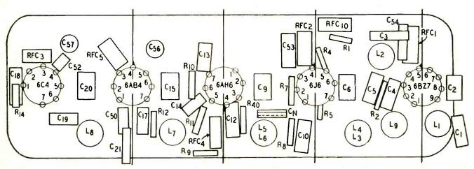
Fig. 2—Layout diagram of r.f., mixer, and oscillator stages. Component numbers refer to circuit elements shown in Fig. 1. Note the positions of the terminals on the tube sockets, and the connections between interstage shields and heater pins.
