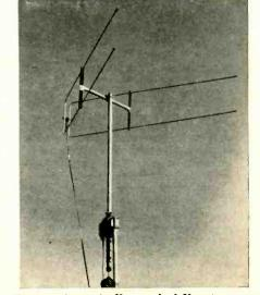
Fig. 4—A vertically-stacked V antenna.
