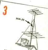
With the Mighty Match you can use a single transmission line between separate high and low channel VHF an.
