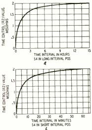
Fig. 3-Approximate long- and shortinterval calibration curves for use with a linear timing-control potentiometer.
