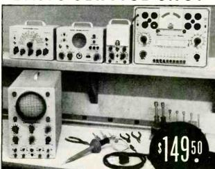
This group of instruments represents a typical combination of basic test equipment required for Radio and TV service work. Here is emphatic proof of the tremendous economy offered only by Heathkits. Seven basic equipment items for less money than the price quoted for a single commercially available instrument such as a general purpose oscilloscope. A serviceman can easily assemble this entire group of instruments in 45 actual working hours.
