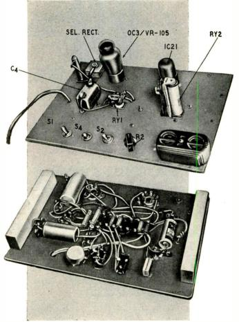
T IS often convenient and sometimes necessary to have a means of turning various types of electrical equipment on or off automatically, after a predetermined time interval. This electronic interval timer does just that, and combines versatility, dependability, and ease of operation with low cost, simple construction, and minimum operating power.
