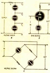
Fig. 3—(a) Neon-lamp voltage divider. (b) A neon lamp as a cathode-bias resistor. (c) Voltage-discriminator circuit.
