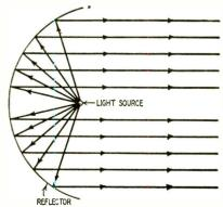
Fig. 10—l'arabolic reflector collects light rays emitted by source and radiates them in unidirectional parallel rays.
