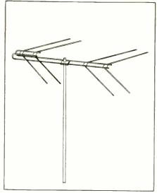
Fig. 6—Four-element "trombone" antenna. Both sets of elements may be adjusted to vary the terminating impedance, and the directivity of the antenna.
