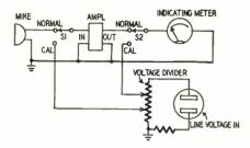
With switches S1 and S2 in positions shown, the amplifier is ready for normal use. To test its gain, S2 is thrown to CAL. The meter measures a relatively high voltage from the line voltage divider. This reading is noted. Now S2 is returned to NORMAL and S1 is switched to CAL. This feeds a small a.c. signal to the amplifier. If the amplifier gain is correct, the meter will show the same reading as before.
