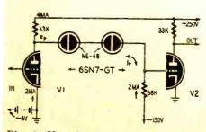
Fig. 4—Neon-lamp interstage coupling circuit for audio and d.c. amplifiers.
