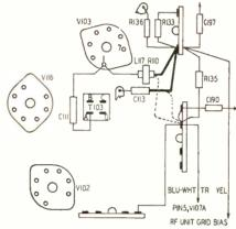
Fig. 1-Wiring changes in RCA KCS38.
