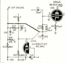
Fig. 2-Schematic of circuit changes.
