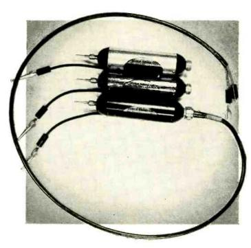
Three types of oscilloscope probes used in TV test work. (Top) Crystal-demodulator signal-tracing probe; (center) low-capacitance high-impedance 10-1 voltage-divider probe; (bottom) 100-1 capacitance-divider high-voltage probe.
