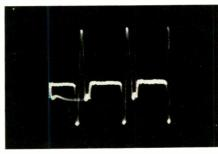
Fig. 6—(Top) Distortion in horizontal yoke current. Nonlinearity shown would compress left side of picture. (Bottom) Negative undershoot in high-voltage waveform drives the plate of the horizontal-output amplifier negative. This may generate Barkhausen oscillations, causing vertical bars on screen.
