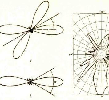
Fig. 3-Directivity pattern of doubleantenna. Note the strong forward lobe, and the relatively narrow minor lobes at intervals of approximately 45°.
