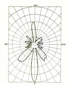
Fig. 5—Higher forward directivity obtained with vertically-stacked V antenna.
