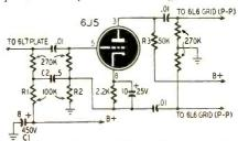
Adding R1 and C2 to the circuit increases the gain tremendously. (See pages 98 and 100, January, 1953, for the theory of this circuit.—Editor) The reactances of C1 and C2 are so low at audio frequencies that R1 and R2 are effectively in parallel. For balanced output from both halves of the inverter, the effective resistance of R1 and R2 in parallel should equal the resistance of R3. So we make R1 and R2 each twice the value of R3.
