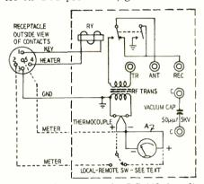
Fig. 1-Diagram of the BC-442-A unit.
