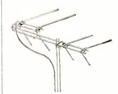
installations to cover u.h.f. The model TV-180 covers all u.h.f. channels and features a uniform gain of 8 db across the band, low voltage standing-wave ratio and 300-ohm impedance. The all-aluminum unit is about 2 x 2 feet and weighs less than 2 pounds.
