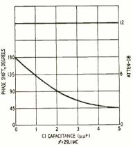
Fig. 3—Phase-shift versus capacitance curves for Pawley bridged-T networks at frequencies of 4.17 kc and 29.1 mc.
