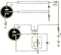
until C can discharge its negative voltage through R. This resistor is shown as a variable element. If, for example, it is reduced, the blocked interval becomes less. Then the average current through V2 is increased. Since V1 and V2 are coupled through a common dropping resistor, the r.f. tube gets less plate potential. As in any self-excited oscillator this means a change in carrier frequency.
