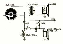
Fig. 3-Schematic of two-way speaker system with Isophon electrostatic unit.
