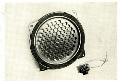
Fig. 2-Isophon electrostatic tweeter. Coil is part of the high-pass filter.
