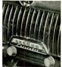
for tuning is completely automatic. Ideal performance is yours with this custombuilt, 7-tube, 3-gang radio. Assures top
