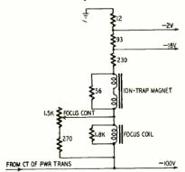
Fig. 3—Focus-control and negative-d.c. supply circuits in 630-type TV receivers.
