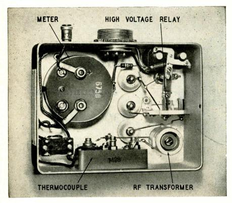
Underside of the antenna relay unit, with cover removed to show components. The resistor between ground and the REC terminal is not used in all models.
