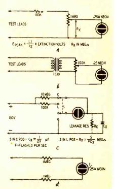
Fig. 6—(a) Simple slideback voltmeter. (b) Neon-tube output indicator. The transformer steps up low voice-coil volttages to the striking potential of the tube. (c) Combination capacitance-leakage-resistance checker. (d) Circuit tester.
