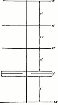
Fig. 5-Dimensions of channel-49 Yagi.
