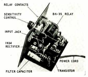
HE HEART of this tubeless remote-control relay is the new Raytheon CK-722 junction transistor. It will operate garage-door openers, lighting circuits, or alarms, or will perform almost any type of switching operation. The relay can be operated by a photocell, radio signal, thermocouple, or any device that will furnish .00025 watt of power.
