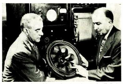
New RCA LC-1A high-fidelity speaker shown here by Dr. H. F. Olson (right) and John Preston, co-developer, has irregularly spaced deflector domes mounted on its 15-inch main diaphragm to break up symmetrical standing-wave interference patterns and flatten the frequency response.
