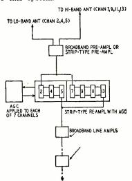
Fig. 2—A composite dual-antenna community TV system. Preamplifier feeds "re-amplifiers" with individual a.g.c. The input lines are shown at top of channel units; outputs at the bottom feed broadband amplifiers which supply signals to the distribution system.
