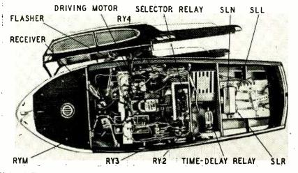
This bird's-eye view into the hold of the model cabin cruiser with the deck and superstructure removed shows the layout of the complete radio-control installation.
