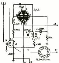
L1 - 8T N°22 ENAM ON SAME FORM 1/2"DIA L2 - 4T OS - L3 = 27MC TANK; L4 - 4T N° 18 HOOKUP WIRE
