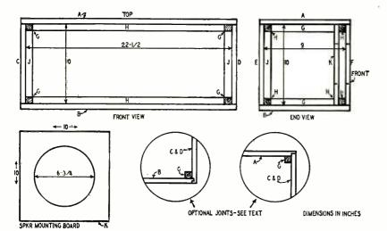
Fig. 1—The construction of a bookshelf-type cabinet for an 8-inch speaker. The  $\frac{3}{4}$ -inch blocks are used in all corners except where sides C and D meet front F. JULY, 1953
