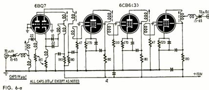
Fig. 5—The SKL "distributed" amplifier. Grid and plate networks delay signals so that all outputs are in phase.
