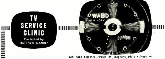
Left-hand foldover caused by excessive plate voltage on the horizontal oscillator in a Synchroguide sweep system.
