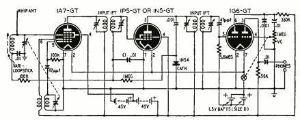
Fig. 1—Schematic of the high-performance portable. The ferrite-core antenna coil, whip antenna, and grid-leak detector give exceptional sensitivity and ample headphone volume without the extra drain of an audio power-amplifier stage.
