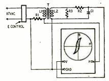
Fig. 7—Equipment setup for checking hysteresis characteristics of iron and transformer core. See text for details.
