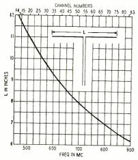
Antennas with thin-wire conductors supported by insulators at the ends are shorter than the free-space dimension because the insulators act as capacitors connected to the dipole ends. The added capacitance causes the dipole to resonate below the design frequency. The added capacitance is called end-effect and must be compensated for by multiplying the free-space constant (5,900) by a decimal constant K. Below about 35 mc, K is approximately 0.95 for most applications.
