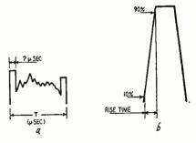
Fig.3—Representative waveforms whose duration may have to be measured. (a) Complex wave. (b) Pulse-waveform display levels for measuring rise time.
