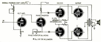
Fig. 5—A combination of balancing arrangements for a Williamson-type amplifier. The adjustable cathode resistor in the phase inverter equalizes the outputs to the driver grids. Feedback from the output-transformer secondary to the driver cathodes helps equalize the push-pull stages. See discussion in the text. Only components essential to the discussion are shown in this schematic.
