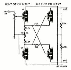
Fig. 3—Cross-coupled phase inverter with cathode balancing potentiometer.
