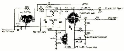
Fig. 1—Delayed keyed-a.g.c. circuits of the late-model Du Mont RA-166, 167, 170, and 171 *Telesets*. The 12AU7 voltage-regulator tube stabilizes the gain of the 6AU6 a.g.c. amplifier against variations in B plus and power-line voltages.
