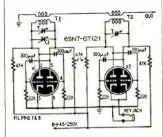
When the unit is used as a b.f.o., the key is opened so V1 operates alone. Its signal beats with the incoming c.w. signal to produce an audible note. The pitch of the note can be adjusted with the variable trimmer.
