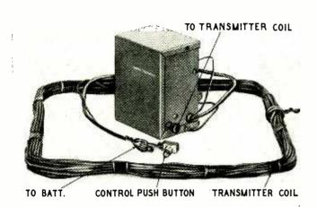
(Above)—The car-transmitter case and loop winding. (Right)—Inside layout of the control-relay housing.
