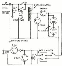
The cycle timer is a chicken-house light timer which I modified to provide half-hour on and off periods. S1 shorts the timer contacts when this feature is not desired.—*Elmer C. Fischer*
