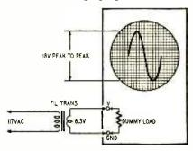
Fig.6—Calibrating theoscilloscopescreen for peak-to-peak voltage measurements. Dummy load should be adjusted so that an accurate r.m.s. voltmeter across the input terminals reads exactly 6.3 volts.
