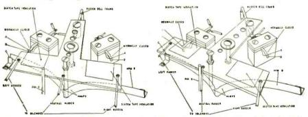
Fig. 4—Two views of the rudder action. When either full right or full left rudder is applied the A,B, switches are opened; at neutral rudder, switch C,D.
