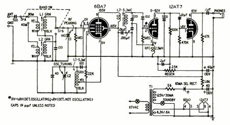
Fig. 1—Schematic of the superhet for the novice and budding ham. A regenerative second detector provides high sensitivity and serves as a b.f.o. for c.w.
