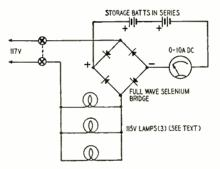
The batteries are charged by the output of the 120-volt, 5-amp full-wave bridge-type selenium rectifier. Charging current is regulated by inserting lamps in the sockets provided for them.
