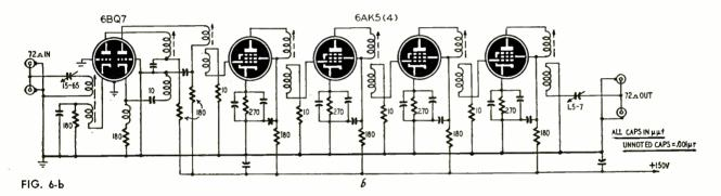
Preamplifiers for community-TV systems generally have low-noise input circuits and voltage gains ranging from about 20 to 55 db. The object is the highest possible signal-to-noise ratio, since the first amplifier stage establishes the minimum system-noise level.
