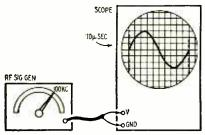
Fig. 4—Equipment setup for calibrating scope screen in time units. One complete cycle of a 100-kc signal is expanded horizontally to occupy 10 scale divisions. Each scale division then represents one microsecond. Higher or lower frequencies may be used for measuring other time units where required.
