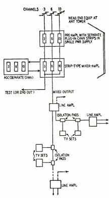
Fig. 3—Block diagram of Philco community-TV antenna distribution system.
