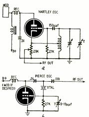
Fig 1—Typical oscillator circuits. (a) Hartley oscillator used in many signal generators. (b) Pierce crystal oscillator preferred for high harmonic output.
