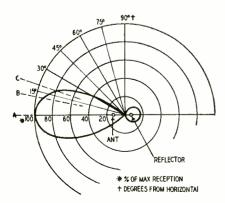
Fig. 1-Vertical-directivity pattern of a horizontal dipole with reflector. The principal lobe offers little discrimination against signals from B and C.
