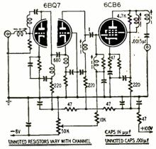
Fig. 7-Philco low-band preamplifier.
