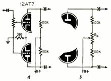
Fig. 4—(a) Basic cathode-coupled phase inverter. (b) Balancing potentiomer inserted in phase-inverter output circuit.
