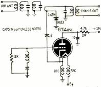
Fig. 2-Typical u.h.f. mixer circuit.
