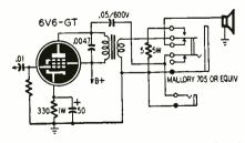
Fig. 2—Safe way to hook up headphones to the output of a TV receiver.
