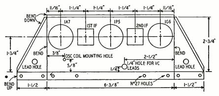
Fig. 2—Suggested layout for the chassis of the portable receiver. Mounting holes for the i.f. transformers and tube sockets will depend on the types used. The chassis can be formed from 22-gauge aluminum or cold-rolled steel.
