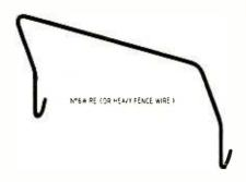
to the approximate shape shown from No. 6 or heavier wire. Use a stiff wire which will not deform under the weight of the chassis.-J. Alibanowicz
