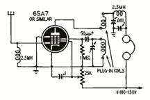
The diagram shows how a 6SA7 or similar converter-type tube can be used as a regenerative detector with one of the control grids used for electronic coupling to the antenna.
