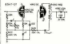
Replace components which are not within the specified tolerances. These tolerances are now being specified in production, and the following new parts numbers have been added: 64A2-16, 60B7-334, 60B7-823, and 60B7-154, for C418, R422, R423, and R428, respectively.—Admiral Radio & Television Service Bulletin
