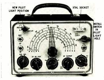
A Heathkit signal generator converted for normal or crystal operation. Most commercial generators can be adapted easily without seriously affecting accuracy of frequency-dial calibrations if additional r.f. wiring is done carefully.
