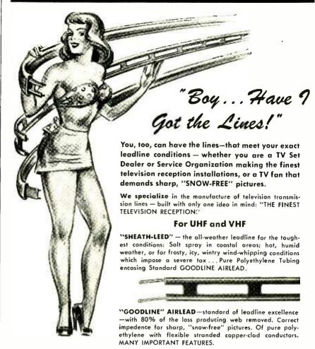
**NEW FULL-WEB "SHEATH-LEED"**— the pure polyethylene of "SHEATH-LEED" and full characteristics of GOODLINE AIRLEAD—but NO PERFORATED WEB. No 20 (7 strand 28) copperweld wire in pure electronic golden clear polyethylene—with a pure silver-gray polyethylene sheath overall—for Maximum Weather Protection.
