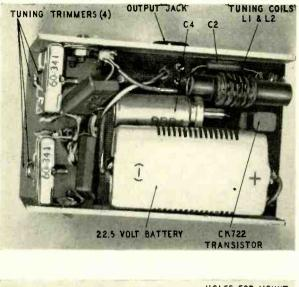
C3 RFC CHASSIS GROUND LEAD HOLES FOR MOUNT-ING ON S1 R2 R3 WINUS BATTERY LEAD
