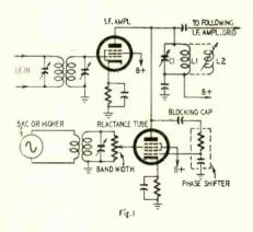
controlling the apparent bandwidth of i.f. amplifier circuits. The circuit in Fig. 1 is for controlling the response of a conventional single-peaked response curve.
