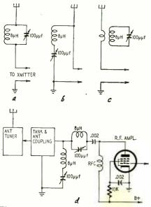
Fig. 3-Various types of antenna traps.
