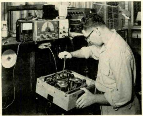
A service technician using special bending tool to set critical mechanical clearance.
