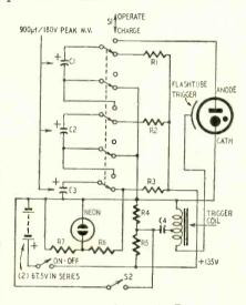
An article in The Radio Constructor, a British publication, describes an electronic photoflash unit using two 67.5volt portable radio batteries in a novel arrangement to supply operating voltage for a flash tube requiring 400-450 volts.
