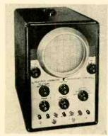
Sensitivities are: vertical-10 millivolts per inch; horizon-tal-150 millivolts per inch. The vertical plates are 24 volts per inch, and the horizontal plates are 26 volts per inch. The input impedances are: vertical amplifiers-5 meg, 26 µµf; horizontal amplifiers-5 meg, 31 µµf; vertical and hori-zontal plates (direct)-4.7 meg. 16 µµf; accelerating potential -2,200 volts. Sweep rates are from 25 cycles to 50 kilocycles.
