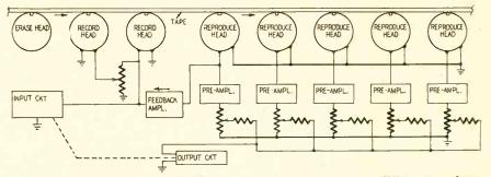
Fig. 2—Sound from input circuit is recorded at two different points. Separate preamplifier volume controls permit a gradual decay of sound.
