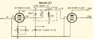
to oscillate within the range of 2 to 3 mc and cause raspy sound and a beat pattern in the picture. Two replacement capacitors are rec-
