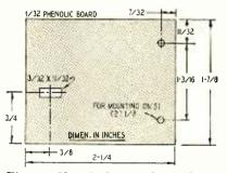
Fig. 4-Chassis layout dimensions.
