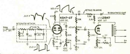
Fig. 4—Multivibrator-type oscillator used in Westinghouse chassis V-2247-1. RADIO-ELECTRONICS
