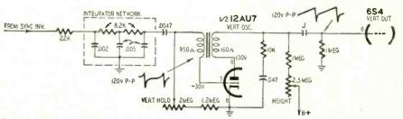
Fig. 3-Integrator network in vertical sweep circuit of Admiral chassis 20A2.
