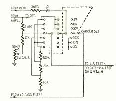
Fig. 5-Diagram of switching circuits.
