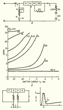
Fig. 1-a—The 4-zone semiconductor. Fig. 1-b—Alpha-emitter bias curves. Fig. 1-c—Circuit variation of Fig. 1-a.
