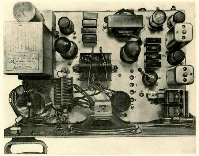
Chassis of typical small-boat radiotelephone.
