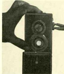
Fig. 10-Shutter at its largest opening.
