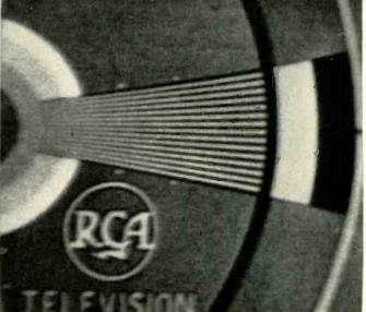
Fig. 2-Lines are properly interlaced.
