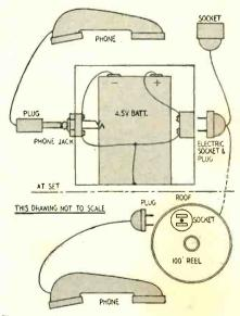
Fig. 5-Carbon-telephone battery box.
