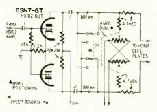
The diagram shows the horizontal output circuit of the Eico 425 scope with the sweep reversal switch added. The signals on the plates of the pushpull horizontal amplifier are 180° out of phase so the sweep changes direction when the plate output leads are reversed by throwing the switch.
