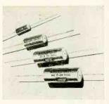
tion of Astron Meteor line of capacitors. X-250 provides high capacitance stability, low power factor, low resonance loss, and high test voltage. The capacitance versus temperature curve of Meteor capacitors is practically flat from  $-40^{\circ}$ C to  $+125^{\circ}$ C, and at  $-65^{\circ}$ C the capacitance decrease with temperature is less than 5%. Type AQ and TQ capacitors are hermetically sealed metaltubular subminiature units de-
