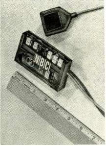
The transistor transmitter. The two "leads" are part of the inductive transmitting loop, which consists of a number of strands of fine wire. The performer can wear it as a belt.
