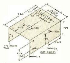
Fig. 3-Layout for the aluminum case.
