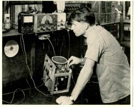
A recorder's electronic circuits are checked with standard eqmipment used for audio and radio.
