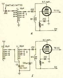
Fig. 1-a—Basic r.f. output circuit. Fig. 1-b—Output-circuit modification. that permits optimum loading, and an antenna resonant at the fundamental frequency. Naturally, shielding and grounding are important, but it will be assumed that these features are adequate, since most of the interference is caused by current that gets out through the antenna wire. Let's see how the marine radiophones stack up.
