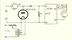
rent. Plate current and amplitude of the r.f. output are controlled by varying the filament voltage.
