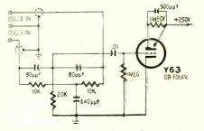
In the usual parallel-T designed as a filter or for the feedback circuit of an oscillator, the constants are selected for maximum possible attenuation at the null frequency and minimum losses elsewhere in the spectrum. In this aplication, the attenuation must be high through the comparatively wide band of frequencies where pulling may occur, so the values are slightly different from those in normal filter and null circuits.
