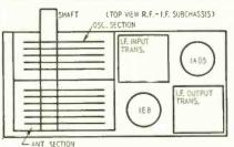
Fig. 3-Lavout of r.f.-j.f. subchassis. scopes within a <sup>1</sup>/<sub>8</sub>-inch hollow length of brass tubing. Total length when extended is 19 inches.
