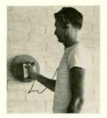
A compact metal detector that will distinguish between metallic iron and other metals such as gold and silver has been developed by Gardiner Electronics Co., Phoenix, Arizona. The unit contains only one tube, a 1R5, and 2 cells. When iron is detected, the earphone signal becomes louder; when other metals are detected, the signal decreases.
