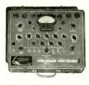
... three toggle switches make it possible to check and compare sections of twinsection tubes at only one setting of selector switch. Transconductance measurements high as 30,000 micromhos with fikered d-c plate, screen grid, and control grid potentials. Precision voltage divider network and switch provides signal voltages of 0.65, 1.3, 2.6, and 5.2 volts peak to peak at a frequency of 5000 cycles. Tubes checked more closely to circuit operating conditions. Better Gm accuracy obtained.
