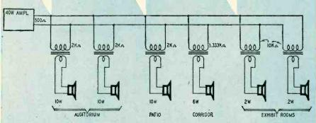
Fig. 1-Diagram shows power distribution in a conventional installation.
