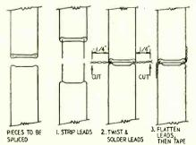
Fig. 3—Splicing 300-ohm transmission line for minimum change in impedance.
