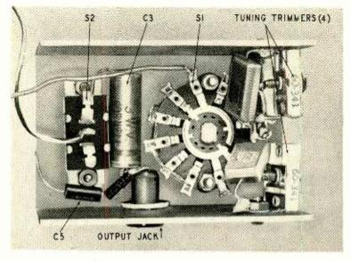
Fig. 5-Components mounted to case.
