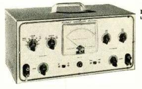
output circuit. The response of the filter is shown in Fig. 3-b. The cathodefollower output is fed simultaneously to an internal v.t.v.m. and to OUTPUT terminals for connecting a scope or a recording oscillograph. The v.t.v.m. is an a.c. type with a push-pull 6AL5 rectifier with a time-constant of 3.3 seconds. The filter and the timeconstant combine to enable the meter to produce accurate indications of peak flutter and wow voltages in the range of 0.5 to 200 cycles.
