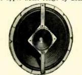
small 3- or 4-inch speaker, mounted either separately or coaxially, as shown in the photo. Make sure the large cone does not hit the mounting straps on low notes. The 2- $\mu$ f coupling capacitor is a low-voltage paper type. Its impedance decreases with frequency, thus feeding the higher frequencies to the 4-inch speaker. At the same time it bypasses the large voice coil for these frequencies.
