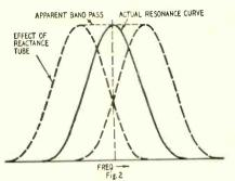
by using the reactance tube to modulate the receiver's local oscillator. Frequency-modulation of the local oscillator results in rapid shifting of the intermediate frequency so the upper and lower side-bands are alternately passed through the relatively narrow i.f. circuits.
