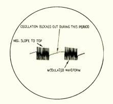
Fig. 2—Oscillogram of oscillator's AM carrier. Modulation exceeds 100%.
