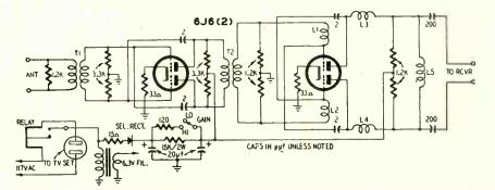
Fig. 1—Schematic of the Electro-Voice 3005FM booster—a wide-band amplifier. SEPTEMBER, 1954 for all recording curves by any of the equalizers designed for magnetic pickups. (This includes the Golden Ear preamplifier which uses a feedback equalizer directly to the input.)
