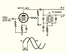
Fig. 1-Oscillator buffer amplifier.
