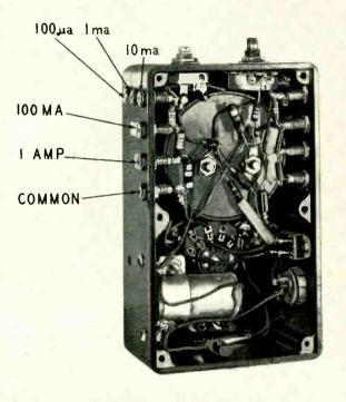
View of the meter's internal wiring.
