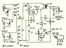
Fig. 1 — Schematic diagram of the transistor AM test oscillator. For stable operation, a 22.5-volt battery is used
