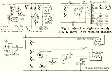
Fig. 3-Schematic of the master unit, used with the power supply of Fig. 1.
