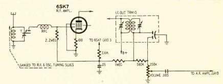
a signal generator, we localized the trouble in the r.f. stage. A resistance check from the grid of this stage to ground showed 100,000 ohms. The normal resistance is 3.7 to 4 megohms as trimmer) had shattered and was partially shorted.
