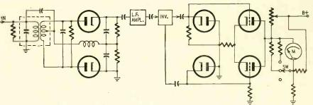
and a pair of limiters. The diodes are fed in push-pull, and their outputs are always positive. For example, in the upper diode electron flow can occur only from ground to cathode, so this element can never go negative. The output triodes are connected in push-push. Their grids are fed out of phase and their anodes are tied together. A push-push stage acts as a doubler, for no matter which triode conducts, anode current flows.
