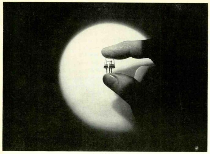
Experimental model of Bell's new high-frequency transistor. It has a cut-off frequency of at least 500 mc and can be used to amplify 2500 independent voices simultaneously.
