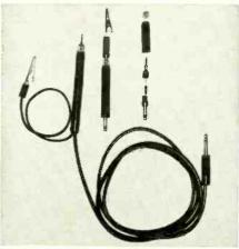
RG-58A/U coaxial cable, with stranded center conductor, meets this requirement admirably. Panel connectors and lead terminations can best be made using a standard phone jack and plug or standard microphone connector such as Amphenol 75-PC1M and the mating plug 75-MC1F.
