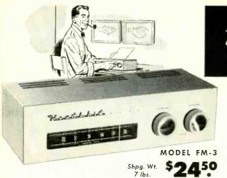
The new Heathkit Model FM-3 features tremendous circuit improvements and brand new physical design. Sensitivity is better than 10 uv. for 20 db of quieting, and it employs a completely modern tube line-up for high gain and stable operation. Incorporates its own power supply, and has provision for low-level or high-level output at low impedance.
