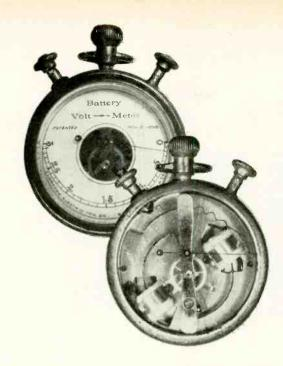
WHAT'S OLD? is the query the instrument to our left brings up. The pocket test set is more ancient than we might imagine, to judge from the patent date (1898) printed on this meter which is apparently intended for checking 1.5-volt dry and probably 2-volt storage cells. Not only is it a pocket job, but is built into a watch case with stem and ring for attaching to a chain.
