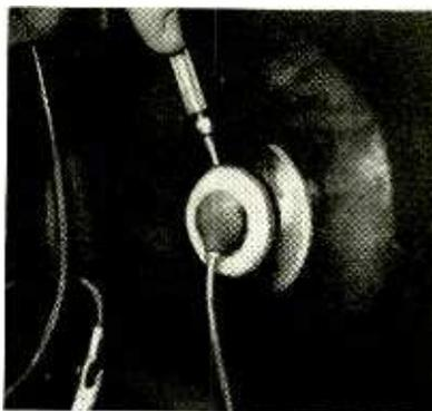
The discharger is simple to use. First, fasten the alligator clip to any point on the TV chassis as in the photo. Then, with the test prod, ground the high-voltage lead at the point where it fastens to the picture tube. The length of nail may be pushed under the rubber cup (if present), thus contacting the picture-tube button. If the set uses a voltage-doubler circuit, discharge both capacitors as an added precaution.
