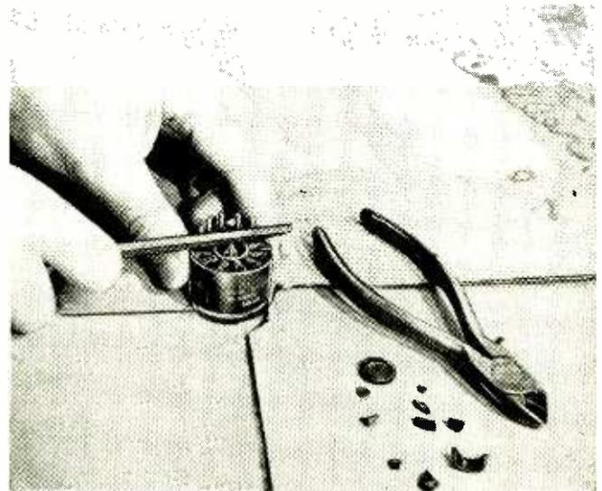
Devacuuming picture tube. Tiny hole filed in exhaust tip lets air in slowly and sounds like leak in tire or a balloon.
