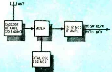
Fig. 1—Block diagram of the 20-40-mc crystal-controlled converter.
