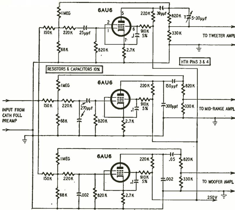
NOTE: When purchasing parts for this circuit, use parts list for Fig. 1 and multiply the number of individual components by the number of channels in the system. Some capacitors are omitted in the tweeter and woofer channels. See text.
