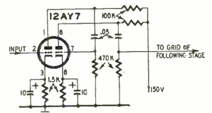
Fig. 2—Two-stage, R-C-coupled triode amplifier.
