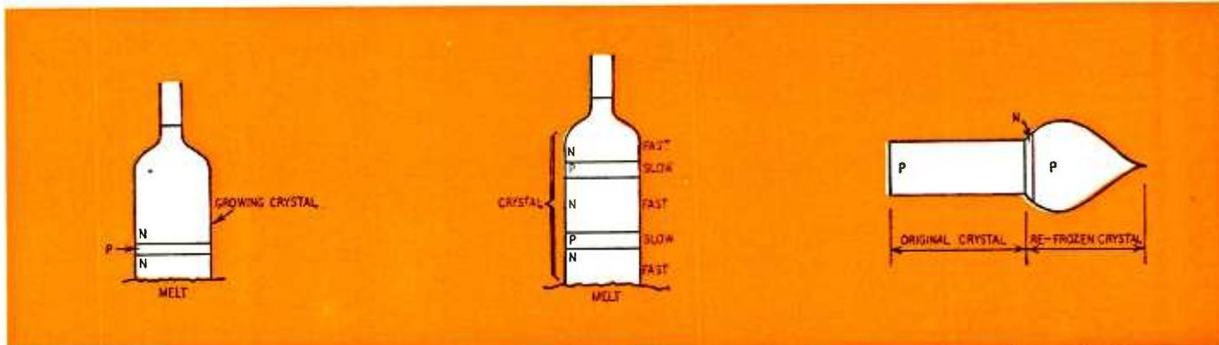
Fig. 2—A grown n-p-n sandwich suitable for transistors.
