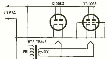
Fig. 1—Recommended test setup for aging tubes for vtvm's.
