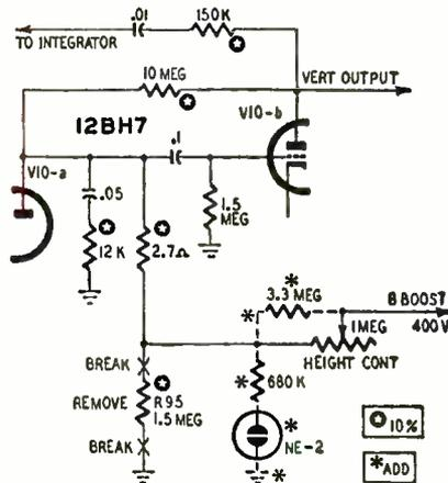
Fig. 4—Bypass action is combined with primary voltage-regulator action in this Olympic C21BD35 modification.
