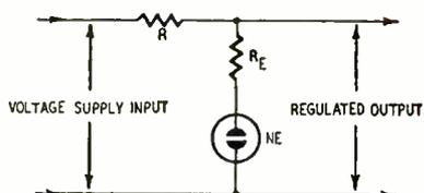
Fig. 3—Typical neon voltage-regulator circuit.
