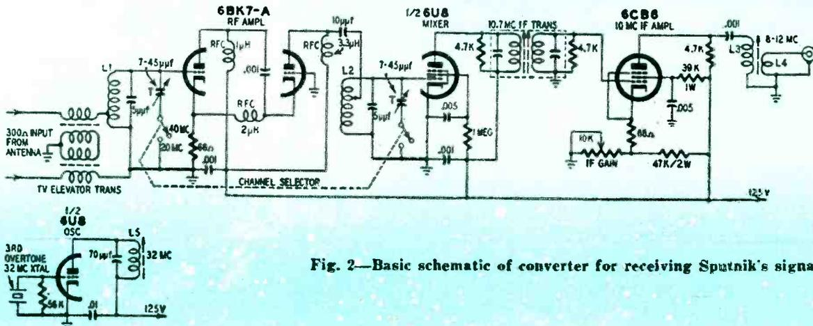
Fig. 2—Basic schematic of converter for receiving Sputnik's signals.
