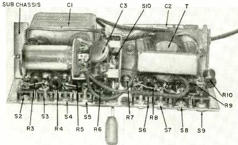
Top view of the timer chassis, showing subchassis assembly.
