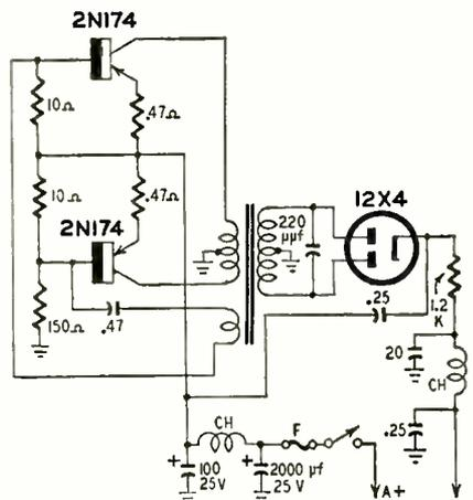
Fig. 10—Transistorized power supply replaces familiar vibrator.
