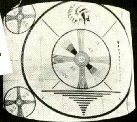
Let's look at this problem: When the fold-over occurs at the right side of the picture, the trouble usually originates in the horizontal discharge or output circuits. Look for the following possible causes:
