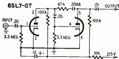
Fig. 4—Standard preamp circuit.
