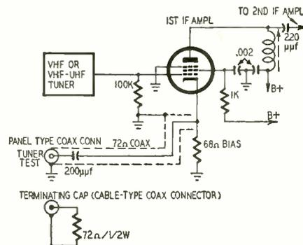
Diagram shows how tuner-test cable is connected in the meter for feeding an if signal into a receiver.
