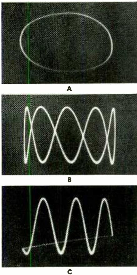
Fig. 4—Calibration, scope patterns: a—60 cycles; b—300 cycles; c—300 cycles at 100-cycle sweep.
