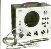
Sep. hi-gain RF & lo-gain audio inputs. Special noise locator. Calibrated wattmeter.
