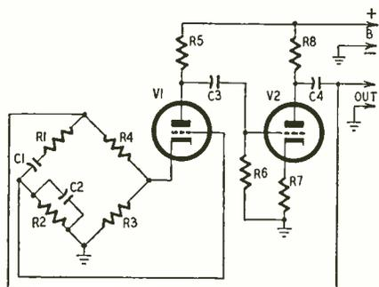
Fig. 1—Basic Wien-bridge oscillator circuit.
