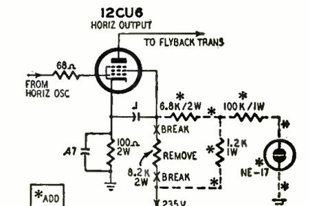
Fig. 5—Simple bypass action removes pseudo Barkhausen interference in an Emerson 120257-D.
