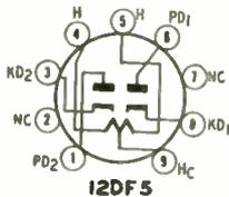
at 12.6 volts, 450 ma or 6.3 volts, 900 ma. It is manufactured by Sylvania.
