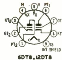
The triode units are isolated by an internal shield having a separate base-pin terminal. Operating characteristics, when used in Class-A1 amplifier service are:
