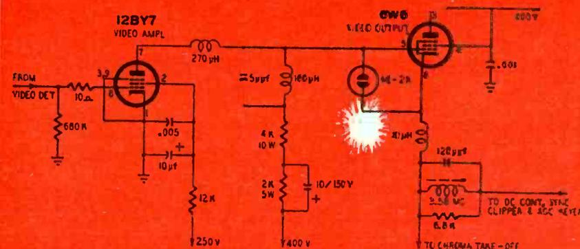
Fig. 2—A neon lamp used as an amplitude limiter and grid-bias regulator in a color set's video amplifier.
