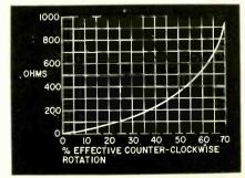
Fig. 3—Taper of pot in meter leg of zero-adjust circuit.
