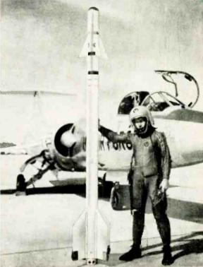
Fig. 6—The Sidewinder infraredguided air-to-air missile. The detection equipment is all in the nose, above the black band.
