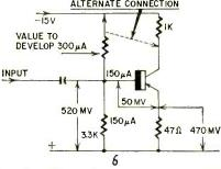
Fig. 11—How the use of an emitter resistance also aids the stabilizing problem by allowing the use of a practical value of base-to-ground resistance.
