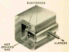
field. The effect is the same as if an infinite number of copper wires, with their ends contacting the front and rear electrodes, were pushed through the space between the magnets. Current is taken from the electrodes.
