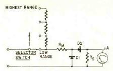
Fig. 6-Typical ac volts circuit.
