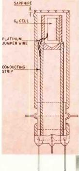
Fig. 4—Cross-section of the detector in Fig. 3.
