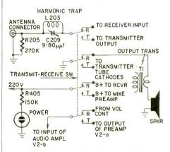
2 — Transmit-receive switching circuits of the CB-1.
