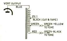
Fig. 3—Correct connection for a Thordarson 26855 replacement vertical output transformer in a Crosley G17TOMH TV receiver.
