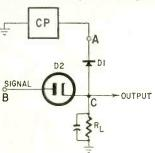
CP, so it does not conduct. At 3 µsec, a signal pulse (2 volts positive) is impressed. Since CP is zero at the time, it constitutes forward bias for D1. Thus the next CP causes a large reverse current through D1 and RL. With a
