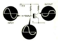
Fig. 8—Relationship between distortions due to base input resistance and nonlinear amplification.
