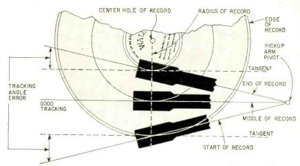
How tracking error is measured
