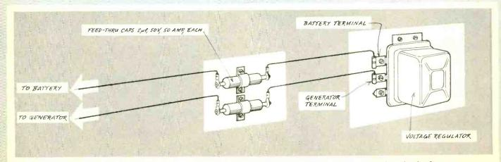
Fig. 1—Coaxial capacitors on the voltageregulator leads stops the popping often caused by arcing breaker contacts. Atthough
