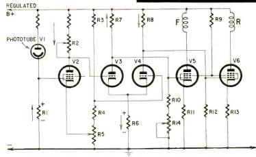
Fig. 10—Circuit of side register control CR7505-S119.
