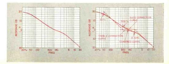
Fig. 2 (right)—The curve of Fig. 1 repeated to show how it consists of two elements, and the design frequencies for those elements.
