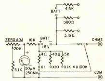
Fig. 2—Another common olummeter circuit. The 4- and 40-ohm resistors are usually the first ones to be damaged by overload.
