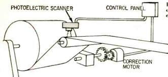
Fig. 2—Basic operation of G-E side register control systems.
