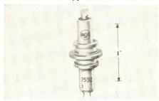
has a maximum plate dissipation of 2.5 watts and can be operated at frequencies up to 1,000 mc and higher. In a typical cathode-drive circuit having a bandwidth of 5 me and operating at 800 mc, the 7552 has a power gain of 18 db and a noise factor of about 8.5 db. The tube's heater is rated at 6.3 volts at 225 ma.
