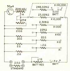
Fig. 6 — Semi-precision ohumeter is somewhat easier to build than the unit shown in Fig. 4.
