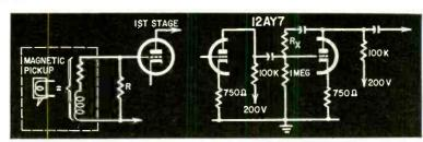
Fig. 7—For some magnetic pickups this arrangement will give the treble or high-end equalization.
