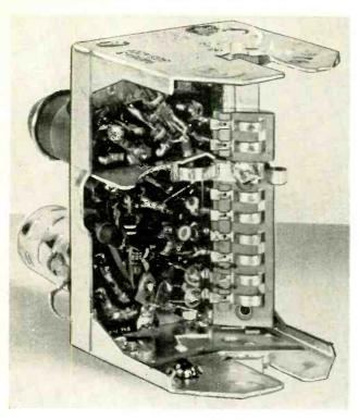
Bottom view of the Guided - Grid tuner with cover and turret removed to show the tuner's printed circuit board.
