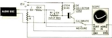
Fig. 5—Setup to measure the input base impedance with different series base resistors, on a sinusoidal current basis.
