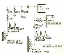
Fig. 3—Horizontal and vertical retrace blanking used in the G-E U4 chassis.
