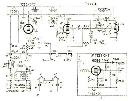
Fig. 1-a—Circuit of the Standard Coil vhfuhf tuner; b—test circuit replaces if strip.
