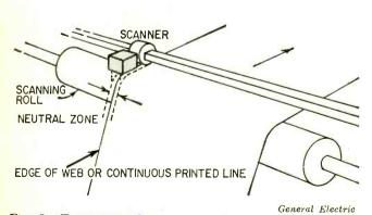
Fig. 8—Two-point side register control system.
