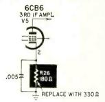
cure called for replacing cathode resistor R26, 180 ohms, with a larger value, 330 ohms. The added bias permits a more normal input to the video detector from the third if amplifier .-Phillip Monroe
