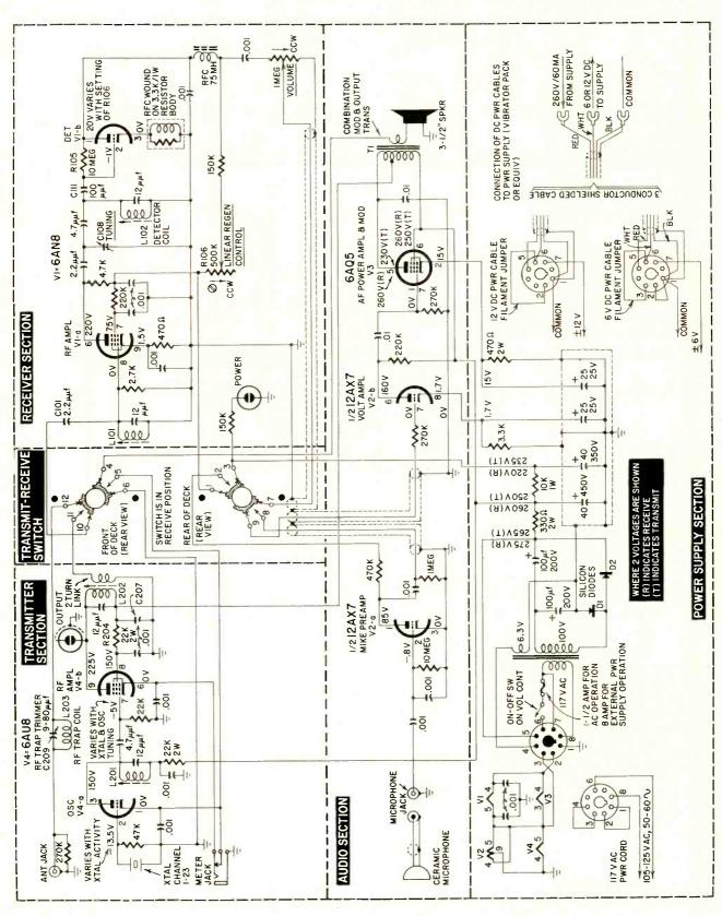
Fig. 1—Circuit of the Heathkit model CB-1 Citizens-band transceiver.
