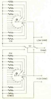
O SI & S3 ARE SIMPLIFIED DRAWINGS OF 18 POINT RANGE SWITCHES IN EICO 1100
