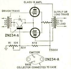
ply well-regulated bias to the class-B amplifier's cathode. The cathode voltage will be equal to the bias voltage, which should be adjusted with R1 for the particular tube being used. The transistor should be bypassed by a  $1-\mu f$  capacitor (dashed lines) for hi-fi applications.—Bendix Semiconductors
