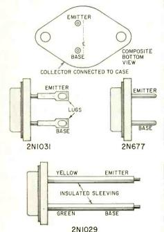
transistors can switch up to 1,000 watts, and have other applications such as power supply regulators, magnetic clutches, relay replacements, power amplifiers, motor control, etc.
