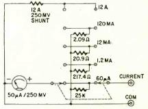
Fig. 5-Special circuit used to prevent contact resistance errors. The 2.09-, 20.9-, and 217.4-ohm resistors are frequently damaged.
