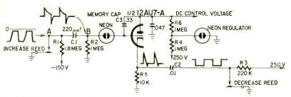
Fig. 5—Partial circuit of Magnavox remote control showing memory section
