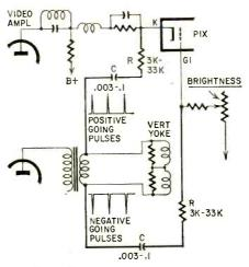
Fig. 4—R-C network adds retrace elimination to a Transvision WRS-3.
