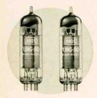
6BQ5 Nine pin miniature power for low power requirements. Two in push-pult deliver up to 17 watts.
