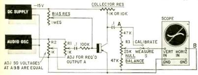
Fig. 1—Using scope balancing method to measure transfer distortion of unloaded transistor stage.
