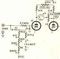
Fig. 3—In this vtvm ohmmeter circuit the 9.75-ohm resistor is normally the only one that burns out.
