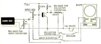
Fig. 7—Measuring input current distortion and output distortion with sinusoidal input voltage.
