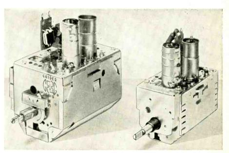
Miniature TV-tuner with Guided-Grid Neutrode circuit is on the right. It outperforms previous standard-sized version,
