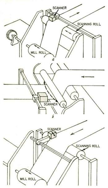
Fig. 7—Three kinds of side register controls: a—pay-off—for guiding a web entering a processing machine; b—mid-line—for guiding a web in the middle of a processing line; c—wind-up—for guiding a web at the exit end of a processing machine.
