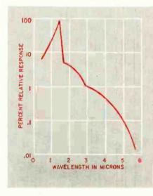
Fig. 5—Spectral response of a gold-antimony doped germanium infrared detector.
