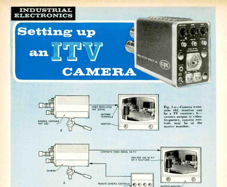
NDUSTRIAL television is the "seeing eye" of industrial electronics; many automatic operations depend on the remote viewing facilities of closed-circuit TV. A number of processes can be monitored from a single central control point with industrial television, and controlled from the same point with industrial electronic equipment.
