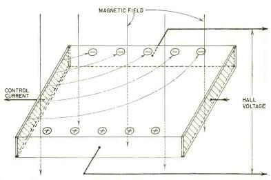
Fig. 1—Basic action of a Hall-effect device. The electrons supplied by the control circuit are deflected by the magnetic field to one side of the conducting slab. This leaves an excess of positive charges on the opposite side, thereby causing a voltage known as the Hall voltage, across the slab.
