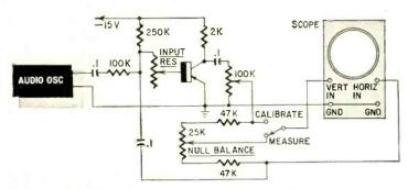
Fig. 6—Measuring input-to-output distortion for voltage input with sinusoidal current.
