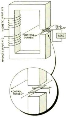
Fig. 2—Typical 2-coil magnetic circuit.
